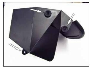
12. Remove the three mounting grommets from the factory air filter housing and install them into the K&N® heat shield where shown.
