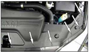
2. Remove the 14 push clips that secure the upper core support plastic cover and then remove the cover from the vehicle.
