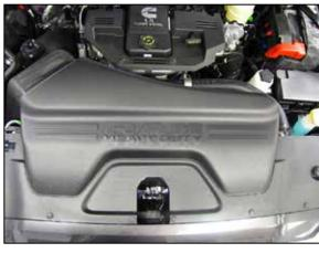
17. Reinstall the factory core support cover and secure with the factory retaining clips.
