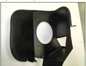
11. Install the provided edge trim around the heat shield as shown, some trimming of the edge trim will be necessary.
