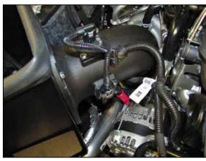
14. Install the intake tube assembly onto the turbo inlet and into the heat shield. Secure the tube with the provided hose clamp and hardware. Reconnect the air sensor electrical connection.
