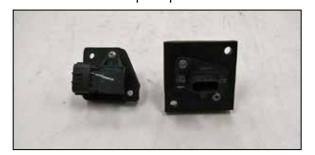
8. Remove the air sensors from the factory housing and install them into the K&N® sensor adapters using the provided hardware.
