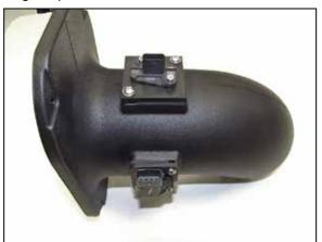
9. Install the two air sensor assemblies into the intake tube using the provided hardware. Be sure the top sensor is installed in the correct direction. The opening of the sensor should be towards the filter end of the tube.
