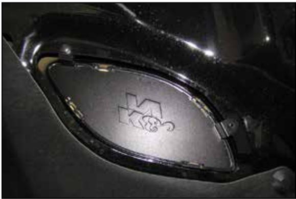
18. Install the provided block off plate and secure with the factory bolts from the previous step.
