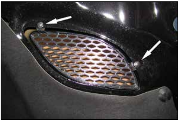
17. During wet conditions on Dodge vehicles to minimize water intrusion to the intake system, remove the two bolts that secure the heat extraction gill to the hood. Do not remove the grill.
