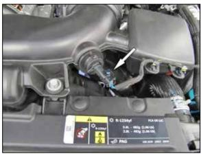
2. Disconnect the inlet air temp electrical connector.
