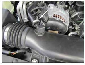
3. Disconnect the crank case vent line.
