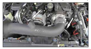
18. Reconnect the crank case vent line onto the quick connect fitting and reconnect the inlet temp sensor electrical connector onto the temp sensor.
