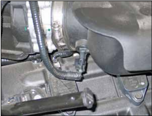
3. Disconnect the inlet air temperature sensor electrical connection.
