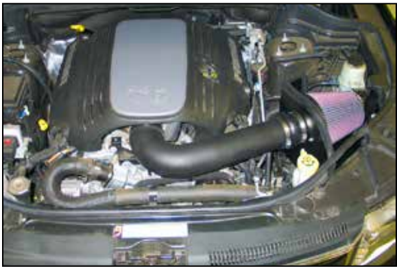
29. Reconnect the vehicle's negative battery cable. Double check to make sure everything is tight and properly positioned before starting the vehicle. 30. It will be necessary for all K&N® high flow intake systems to be checked periodically for realignment, clearance and tightening of all connections. Failure to follow the above instructions or proper maintenance may void warranty.
