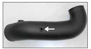
21. Install the provided grommet into the K&N<sup>®</sup> intake tube as shown.
