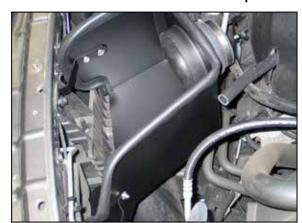
19. Install the heat shield assembly into the vehicle and secure with the bolts removed in steps #17 and 18. Do not completely tighten at this time.
