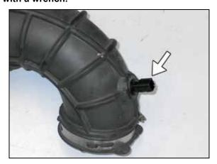
23. Remove the inlet air temperature sensor from the stock intake tube. **NOTE: Take care removing the sensor as it is very fragile.**
