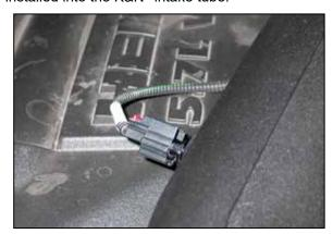
27. Connect the provided inlet temperature sensor extension into the factory wiring harness and then connect the other end to the inlet temperature sensor. NOTE: The vehicle manufacturer uses two different inlet air temperature sensor connections, choose the correct extension harness for the sensor provided by the manufacturer. Secure the harness with the provided tie wrap.
