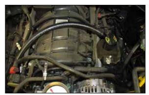
9. Install the K&N CCV hose assembly onto the factory port and position the assembly as shown.
