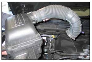
5. Disconnect the factory intake hose from the throttle body, then lift up the air box assembly and remove from the vehicle. **NOTE: K&N Engineering, Inc., recommends that customers do not discard factory air intake.**
