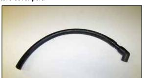
8. Remove the factory 45 deg. elbow from the factory CCV hose assembly. Assemble the K&N® CCV hose, Union and factory 45 deg. elbow as shown.
