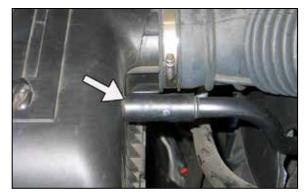
4. Disconnect the crank case vent hose from the air
