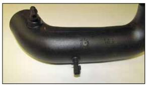
24. Install the inlet air temperature sensor into the grommet installed into the K&N® intake tube as shown. **NOTE: Take care while installing the inlet air temperature sensor as it is very fragile.**
