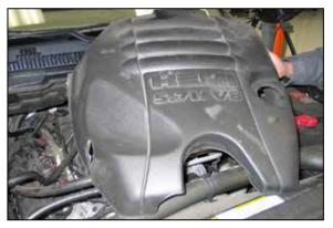
6. Lift up the engine cover to dislodge it from the mounting posts and then remove it from the vehicle.
