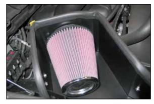
28. Install the K&N<sup>®</sup> air filter and secure with the provided hose clamp.
