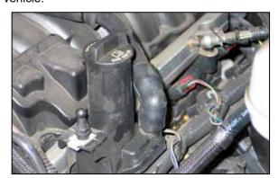
7. Disconnect the crank case vent hose from the valve cover port.
