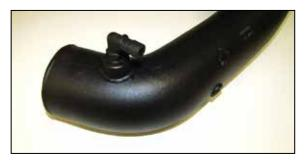
22. Install the 1/4 NPT vent fitting into the K&N® intake tube as shown. NOTE: Plastic NPT fittings are easy to cross thread. Install the vent fitting "hand" tight, then turn it two complete turns with a wrench.
