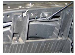
17. Remove the front air box mounting bracket bolt shown. **NOTE: This bolt will used in a later step.**
