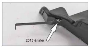
16. Install the heat shield mounting bracket (083103-1A) onto the heat shield using the provided hardware. NOTE: On 2013 and later model vehicles, place the provided spacer between the bracket and heat shield. Do not completely tighten at this time.
