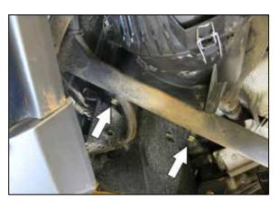
2. Remove the factory air filter housing mounting bolts shown. Save for later install.
