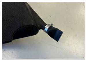
10. Install the supplied "Duck Bill" drain onto the K&N air filter housing and secure with the provided hose clamp.
