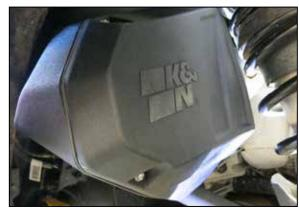
16. Install the air filter housing lid with the provided hardware and gasket.
