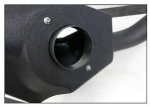
7. Install the provided filter adapter into the K&N air filter housing and secure with the provided hardware.
