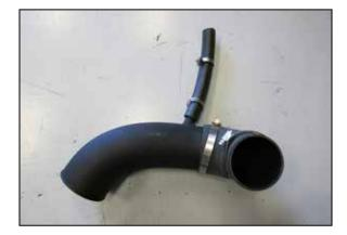
12. Install the provided CCV hose and elbow coupler onto the K&N intake tube as shown.
