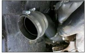
14. Install the provided hump hose onto the intake tube and secure with the provided hose clamp.
