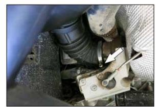
3. Loosen the hose clamp that secures the factory intake tube to the turbo inlet.
