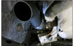
13. Install the K&N intake tube assembly onto the turbo inlet and connect the CCV hose to the engine with the provided hose clamps. Tighten clamps on the CCV hose only. Do not secure clamps on elbow coupler.
