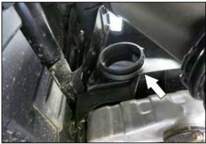
11. Install the fresh air inlet bell into the stock fresh air-pass hole through the body work.
