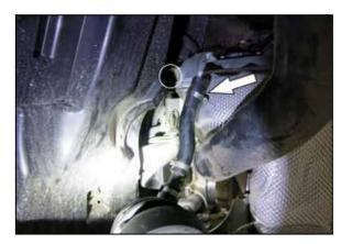
6. Loosen the hose clamp that secures the CCV hose to the engine, remove the complete factory intake system.
