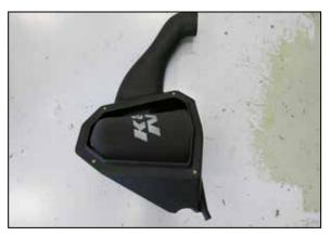
9. Install the air filter into the K&N air filter housing and secure with the provided hose clamp.
