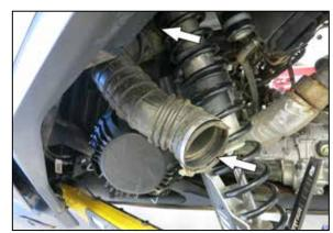
5. Remove the factory fresh air intake duct.
