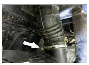
4. Loosen the hose clamp that secures the fresh air duct to the factory air filter housing.
