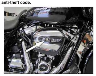
2. Loosen and remove the bolt which secures the decorative filter cover and remove the cover from the vehicle.
