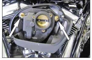
4. Remove the two breather bolts shown and then remove the rear air filter housing from the vehicle.
