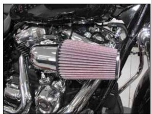
11. Install the air filter onto the intake tube and secure with the provided hose clamp.
