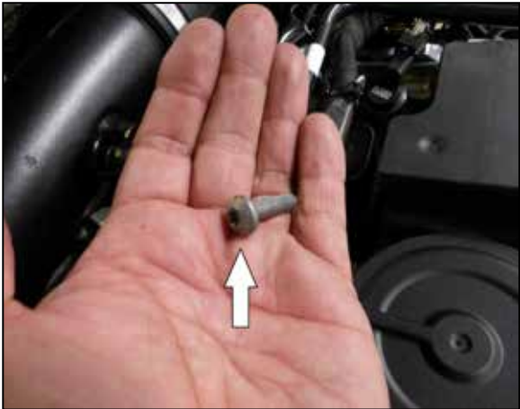
4. Behind the intake tube near the previous step, locate the T30 torx bit bolt, loosen and remove. This is holding in the intake tube.
