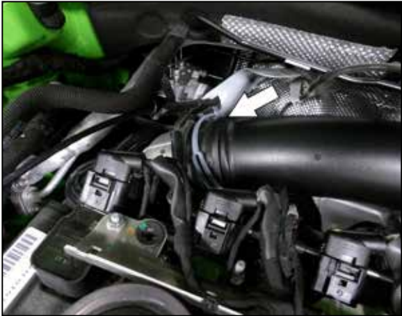
6. With pliers pull back the clamp on the turbo side of the intake tube, and remove the intake tube out of the vehicle.
