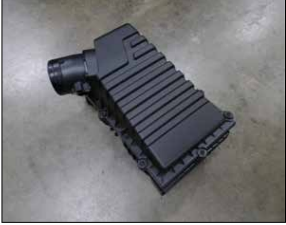
10. Remove the air box out of vehicle. NOTE: K&N Engineering, Inc., recommends that customers do not discard factory air intake.
