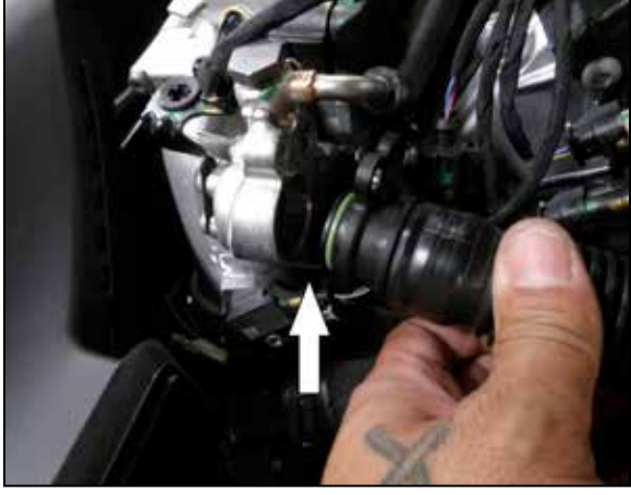
11. On some Models, on the secondary air pump side, loosen and remove the two 5mm allen bolts. Save for later use. NOTE: If your vehicle comes with hose that clamps on to airbox, ignore this step.
