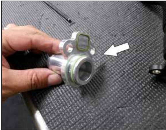
12. With secondary air line removed, remove the two O rings pictures above. Now, install to the new provided Air Fitting. NOTE: If your vehicle comes with hose that clamps on to airbox, ignore this step.
