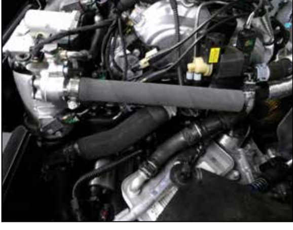
14. Install the air fitting assembly back into the secondary air pump. Secure using Original bolts. NOTE: If your vehicle comes with hose that clamps on to airbox, ignore this step.
