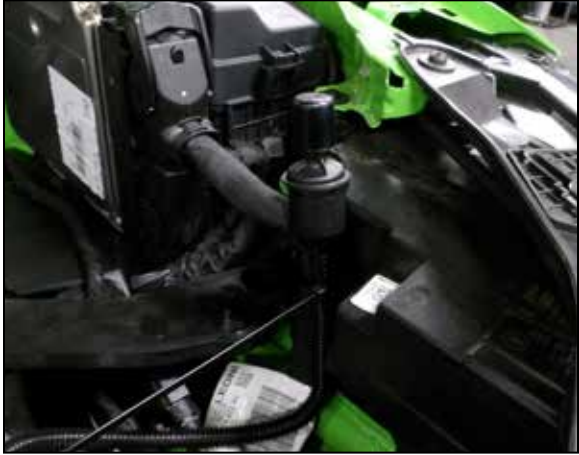
9. Re-locate the transmission vent line to the ECU harness. Secure using provided cable-tie. Trim cable-tie.
