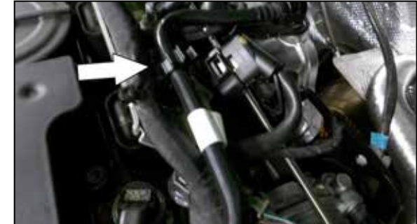
3. Depress the crank case quick connect fitting. Locate the clip holding in the line and pull away from the clip. This will allow for more movement.
