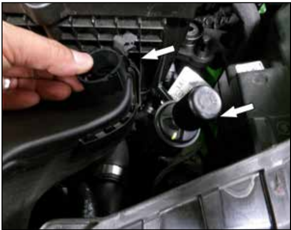
8. Locate the transmission vent line on airbox and remove the harness assembly and put aside.
