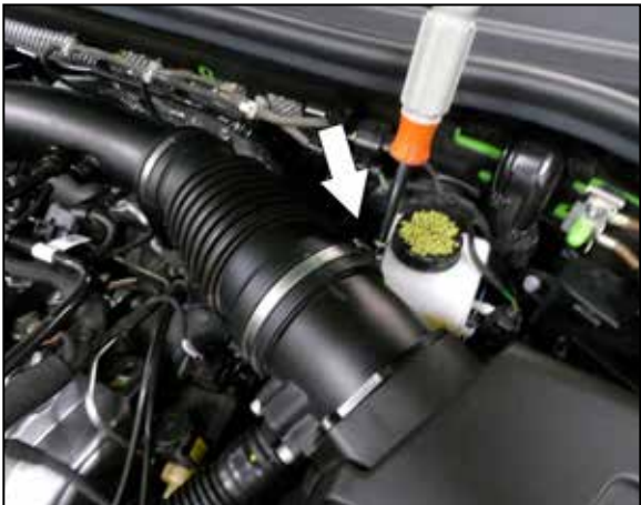
5. Loosen the clamp on the airbox. Pull back the rubber hose away from the airbox.
