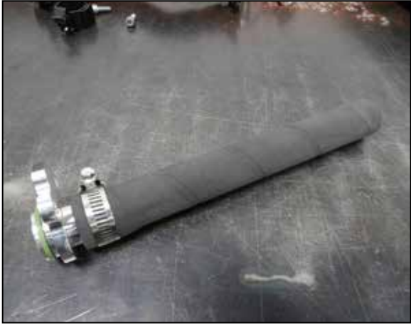
13. With provided hose, With a ruler cut the straight section of hose to 9"L. Now install the hose with clamps onto the air fitting. NOTE: If your vehicle comes with hose that clamps on to airbox, ignore this step.
