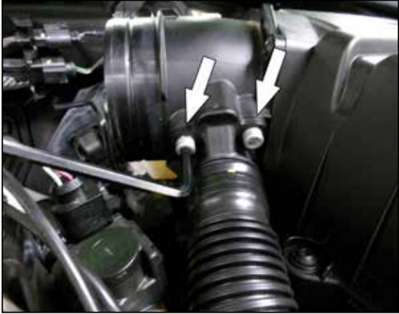
7. On Some models, locate the secondary air line and loosen the two 5mm allen bolts and pull away from the airbox. Other models, remove hose from airbox. See step 22.
