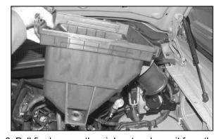
8. Pull firmly up on the air box to release it from the mounting studs, then remove the air box from the
