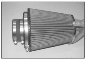
29. Install the filter adapter assembly into the K&N $^{\circ}$  air filter.
