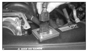
31. Reconnect the mass air sensor electrical connection.
