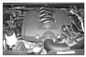
32. Re-install the throttle body cover as shown.
