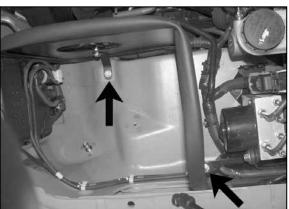
14. Install the heat shield onto the vehicle and secure with the provided hardware.
