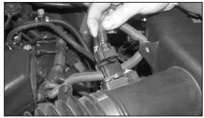
3. Disconnect the mass air sensor electrical connection, then release the wire loom from the air box.
