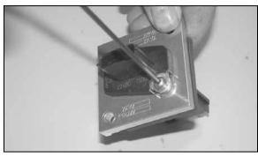
21. Insert the mass air sensor into the mass air sensor adapter and secure with the provided hardware.
