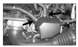
4. Remove the two vent lines from the air intake resonator as shown.
