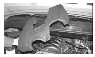
2. Remove the two bolts that secure the throttle body cover, then remove the throttle body cover.
