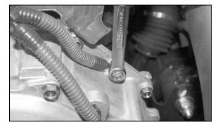
16. Locate the ground wire attached to the engine cam cover and remove the bolt securing it using a 10mm wrench.
