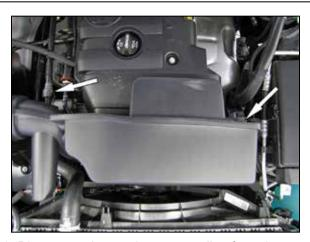
3. Disconnect the crank case vent line from the intake plenum and remove the bolt that secures the intake plenum to the engine. Remove the intake plenum from the vehicle.
