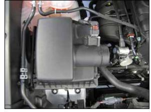
4. Loosen the four bolts that secure the upper air filter housing to the lower housing, then remove the housing and factory air filter.
