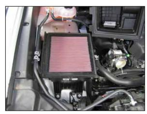
5. Install the K&N® air filter and then reinstall the upper housing and secure with the factory screws.
