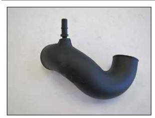
7. Install the provided vent fitting into the into the K&N® intake tube as shown.
