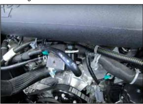
13. Rotate the crank case vent line to line it up with the quick disconnect fitting installed into the K&N® intake tube and then connect the crank case vent.
