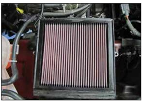
6. Replace the factory air filter with the K&N<sup>®</sup> air filter provided. Reinstall the upper air filter housing and secure with the factory screws.
