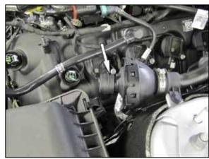
6. Install the provided cap onto the sound drum.
