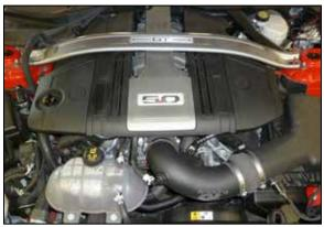
13. Reinstall the decorative engine cover and strut bar, secure with the factory hardware. Reconnect the negative battery cable.
