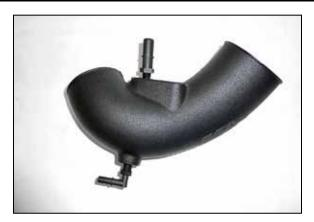
11. Install the provided vent fittings into the K&N® intake tube as shown.
