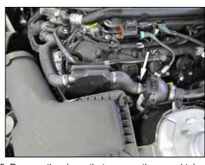
5. Remove the clamp that secures the sound tube to the sound drum and then remove the sound
