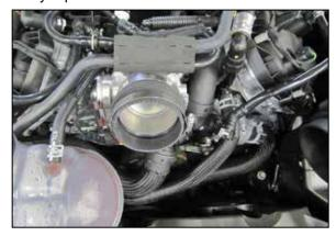
9. Install the provided coupler hose (08698) onto the throttle body and secure with the provided hose clamp.
