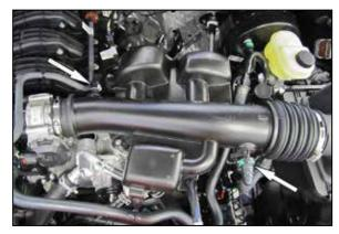
2. Disconnect the two intake vent lines shown.
