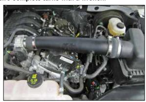
9. Install the K&N® intake tube into the Coupler at the throttle body and then onto the coupler at the air filter housing. Secure the upper air filter housing and then adjust the tube for best fit and secure with the provided hose clamps.
