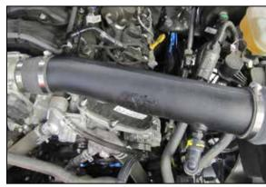
11. Connect the factory vent lines to the quick connect fittings installed into the K&N® intake tube.
