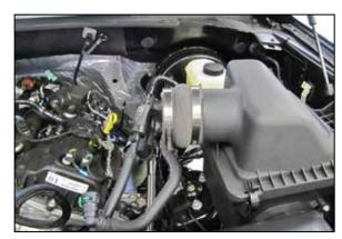
7. Install the provided coupler hose (08639) onto the air filter housing and secure with the provided hardware.
