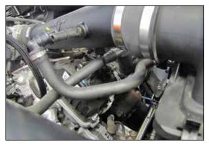
10. Secure the vent hose to the K&N® intake tube with the provided mounting head tie wrap.
