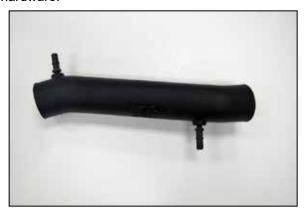
8. Install the provided quick connect fittings into the K&N® intake tube as shown.
