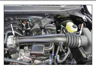
3. Loosen the hose clamps that secure the intake tube, unclip the coolant line and vent hose clip and then remove the factory intake tube.
