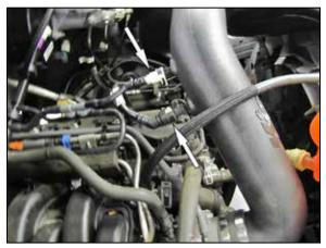
9. Connect the EVAP and crank case vent lines to the quick connect fittings installed into the K&N® intake tube.
