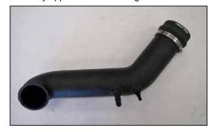
6. Install the Provided vent fittings into the K&N intake tube as shown. Install the provided hump coupler (08683) onto the intake tube and secure with the provided hose clamp.
