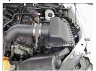
8. Install the K&N® intake tube into the coupler at the air filter housing and then into the coupler at the throttle body, adjust the tube for best fit and then secure with the provided hose clamps.
