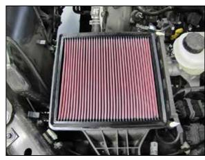
5. Install the provided K&N® air filter and reinstall the factory upper air filter housing.
