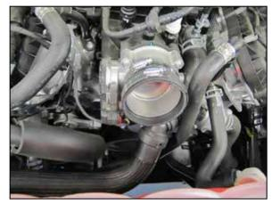
7. Install the provided coupler hose (08615) onto the throttle body and secure with the provided hose
