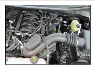
3. Loosen the hose clamps that secure the factory intake tube to the air filter housing and throttle body and then remove the intake tube from the vehicle. NOTE: K&N Engineering, Inc., recommends that customers do not discard factory air intake.
