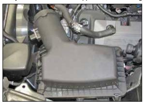
12. Reinstall the upper air filter housing onto the lower housing and secure with the factory retaining clips.
