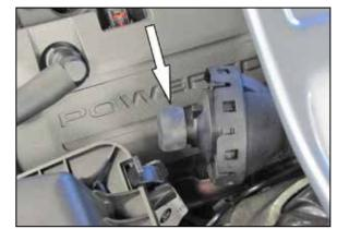
6. Install the provided cap onto the sound drum as
