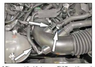
3.Disconnect the Idle by-pass, EVAP vent line and the crank case vent line from the factory intake
