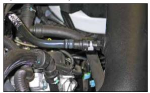
23. Connect the crankcase vent hose to the quick disconnect fitting in the K&N® intake tube.
