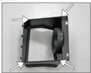
10. Install the two 9" sections of edge trim onto the bottom of the heat shield as shown.
