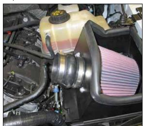
15. Install the provided silicone hose (084057) onto the filter adapter and secure with the provided hose clamp.
