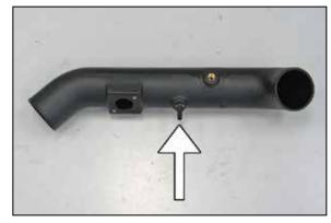
16. Install the provided 3/8" hose fitting into the  $K\&N^{\circ}$  intake tube as shown.
