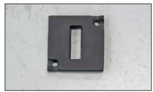
18. Install the provided gasket onto the mass air sensor adapter as shown.
