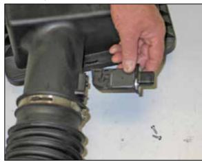
19. Remove the two screws securing the mass air sensor and then remove the mass air sensor from the stock intake tube as shown.
