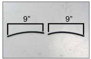
9. Cut the provided edge trim into two 9" sections as shown.
