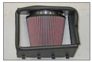
11. Install the K&N<sup>®</sup> air filter onto the filter adapter and secure with the provided hose clamp.
