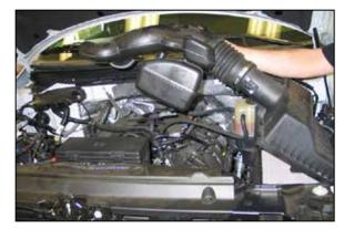
6. Release the three clips securing the upper airbox housing to the lower housing and then remove the intake tube/upper airbox and air filter from the vehicle.
