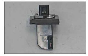
20. Install the mass air sensor into the K&N $^{\! \odot}$  sensor adapter as shown. Secure with the provided hardware.
