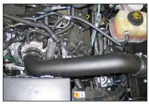
22. Install the K&N® intake tube assembly into the silicone hose at the filter adapter and then into the silicone hose on the throttle body and secure with the provided hose clamps.
