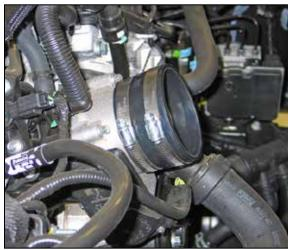
14. Install the provided silicone hose (08630) onto the throttle body and secure with the provided hose clamp.
