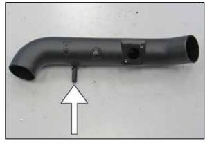
17. Install the provided quick disconnect fitting into the  $K\&N^{\circ}$  intake tube as shown.
