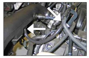
24. Install the provided silicone hose onto the 3/8' fitting installed in the K&N<sup>®</sup> intake tube and then attach the open end to the EVAP check valve.
