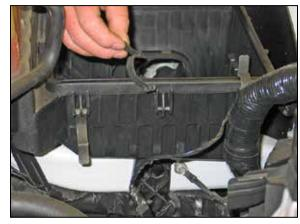
12. Remove the center airbox retaining clip.
