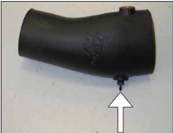
17. Install the provided 3/16" vacuum fitting into the K&N® intake tube as shown.
