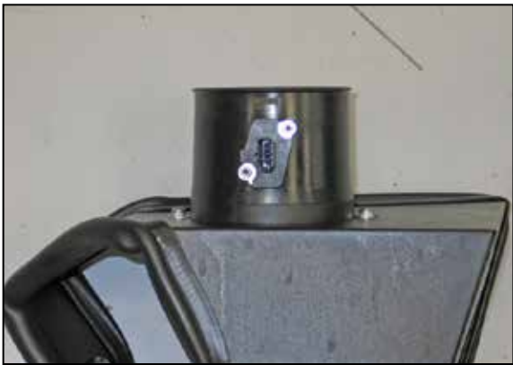
13. Install the mass air sensor into the K&N® mass air sensor housing and secure with provided hardware.
