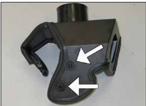
15. Install the factory mounting grommets to the two mounting posts installed on the K&N® heat shield assembly as shown.
