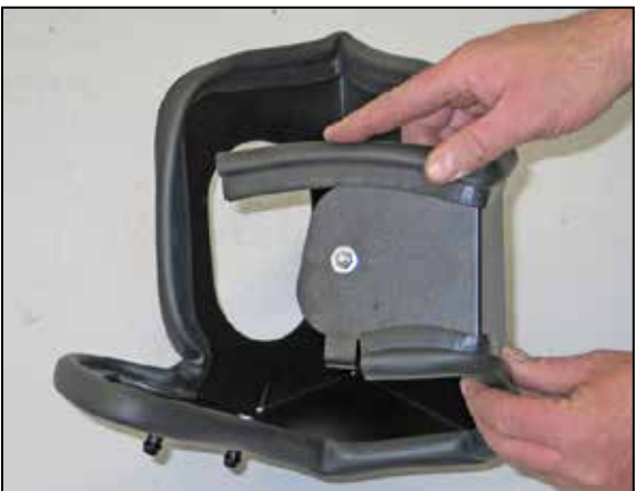
10. Install the provided edge trim onto the heat shield as shown. NOTE: Some trimming of the edge trim will be necessary.
