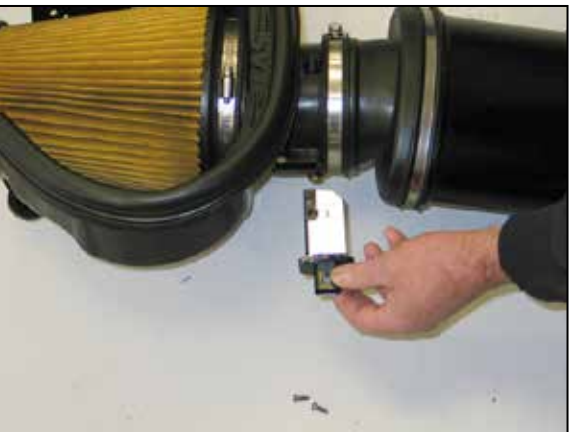
12. Remove the two screws securing the mass air sensor to the factory housing, then remove the mass air sensor as shown.
