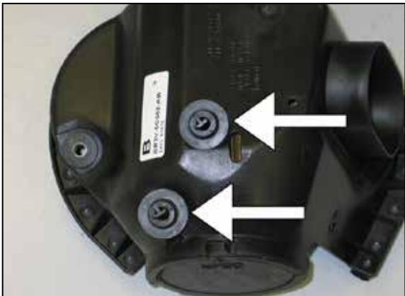
14. Remove the two factory mounting grommets shown from the airbox.
