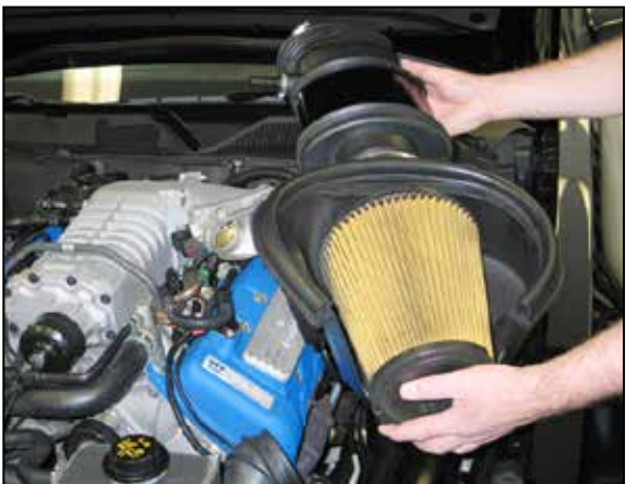
7. Disconnect the intake tube from the throttle body and then remove the complete intake system from the vehicle.
