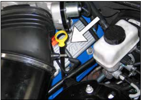
4. Disconnect the vacuum line from the stock intake tube as shown.
