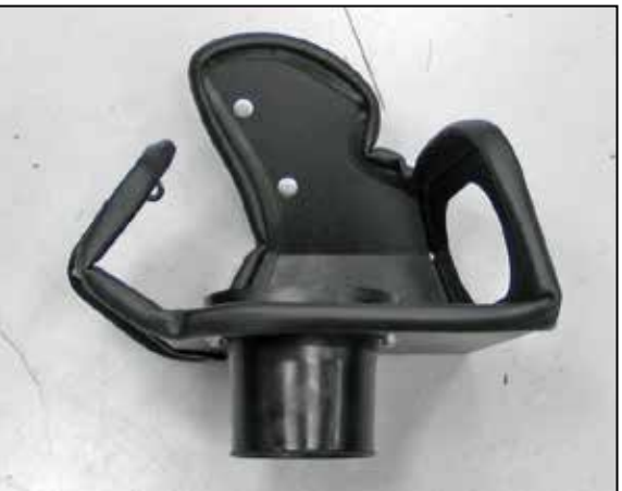
11. Install the mas air sensor into the heat shield, rotate the sensor 180° so the sensor boss is pointed downward, and then secure with the provided hardware.
