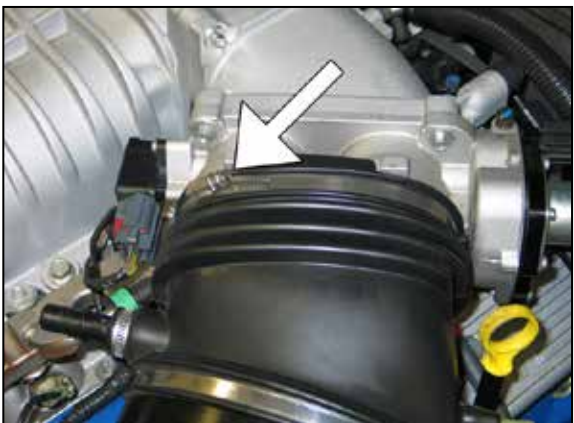
6. Loosen the hose clamp securing the stock intake tube to the throttle body.
