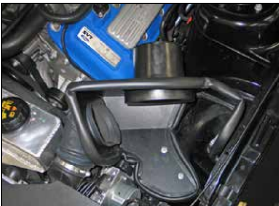
16. Install the heat shield assembly into the vehicle so the mounting bracket aligns with the factory airbox mounting location and the mounting grommets set into the mounting holes. Insert the fresh air duct into the heat shield.
