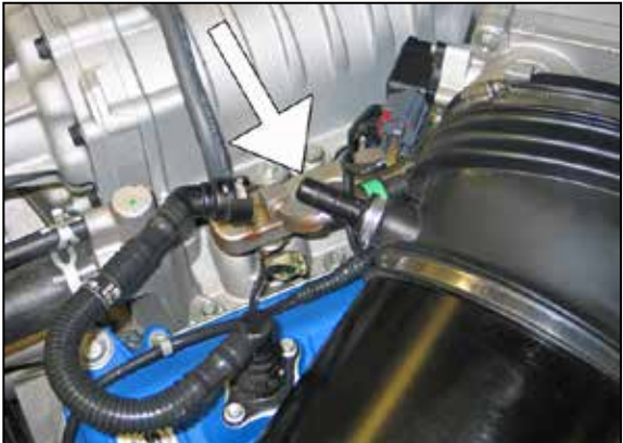
5. Rotate the locking ring and then disconnect the crankcase vent hose as shown.
