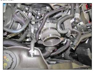
11. Install the provided coupling hose (08699) onto the throttle body and secure with the provided hose clamp.
