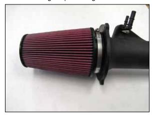
14. Install the air filter onto the end of the K&N® intake tube and secure with the provided hose clamp.
