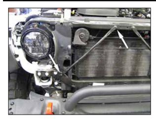
7. Remove the two bolts securing the diagonal core support brace and remove the brace.
