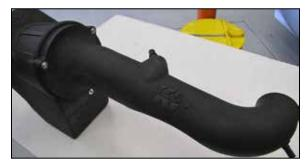
15. Install the K&N® intake tube assembly onto the K&N® airbox with provided hardware. Note the orientation of the K&N® intake tube.
