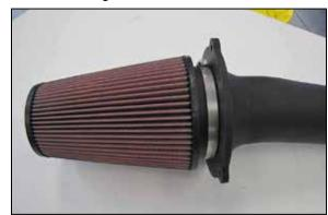
14. Install the K&N® air filter onto the K&N® intake tube.
