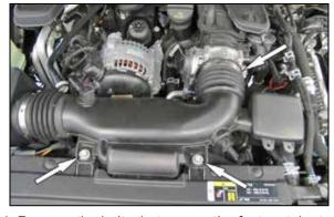
4. Remove the bolts that secure the factory tube to the fan shroud, then loosen hose clamp at throttle
