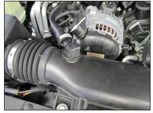
3. Disconnect the crank case vent line.
