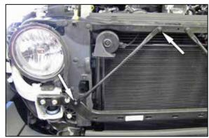
7. Remove the two bolts that secure the core support brace to the core support and remove brace
