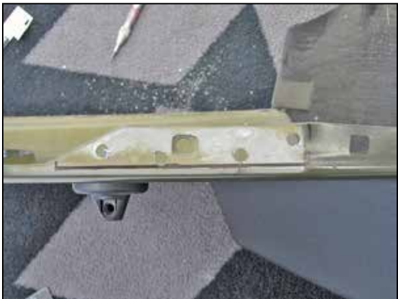
51. Using the provided template, mark the fender where the excess material needs to be removed from the fender.
