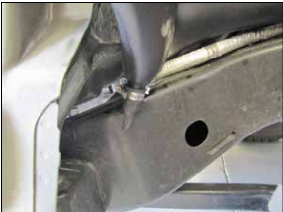
58. Install the duck bill fitting onto the port at the bottom of the corner tube and secure with the provided hose clamp. NOTE: be sure all of the hose clamps securing the corner tube are turned in such a way that the will not interfere with the fender once it is installed.
