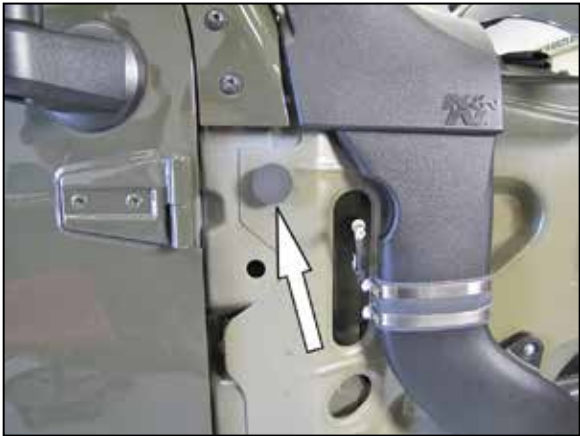
59. Peel the backing of the provided damper pad and then install it as shown on the inner body. NOTE: Be sure all of the hardware is secure before moving to the next step.
