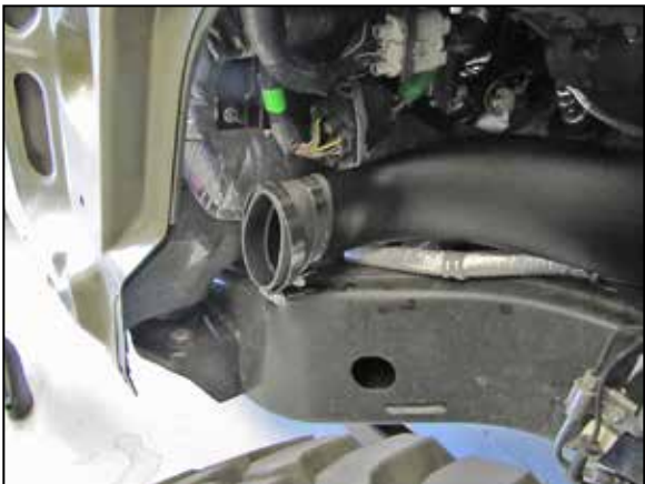
47. Install the provided coupler hose (08711) onto the lower tube and secure with the provided hose clamp.
