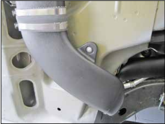
57. Secure the corner tube with the provided sheet metal screw into the hole previously drilled.
