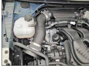
16. Install the K&N® intake tube into the coupling hose at the plenum, align the coupling hose at the filter adapter and then adjust the tube for best fit and tighten all of the hose clamps.
