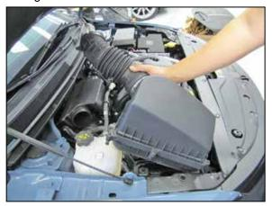
5. Separate the factory intake tube from the intake plenum and then lift up the complete upper air filter housing to dislodge it from the mounting grommets and remove it from the vehicle.
