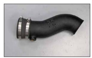
12. Install the provided coupler hose (084091) onto the  $K\&N^{\otimes}$  intake tube fully but do not tighten at this time.
