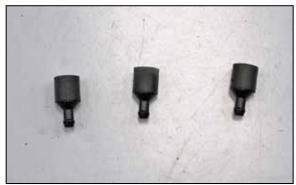
7. Install the three provided heat shield mounting studs onto the rubber mounted studs as shown.
