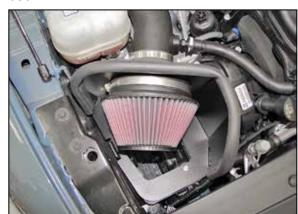
18. Install the  $K\&N^{\otimes}$  air filter onto the filter adapter and secure with the provided hose clamp.
