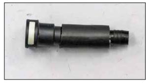
15. Remove the factory quick disconnect fitting from the factory crank case vent hose and install it into the provided vent hose as shown.
