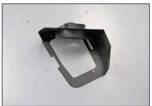
6. Install the provided air filter adapter into the heat shield and secure with the provided hardware.
