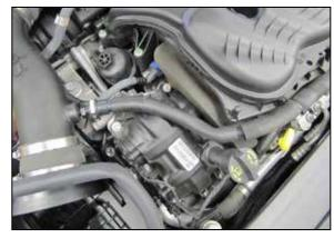
17. Install the crank case quick connect fitting into the factory crank case vent hose and connect it to the fitting installed into the K&N® intake tube.
