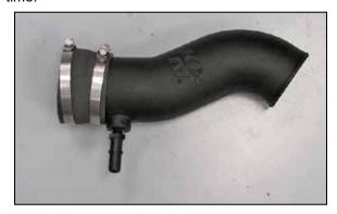
13. Install the provided quick disconnect npt fitting into the  $K\&N^{\scriptsize @}$  intake tube as shown.
