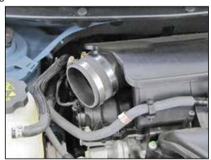
11. Install the provided coupling hose (08690) onto the intake plenum and secure with the provided hose clamp.
