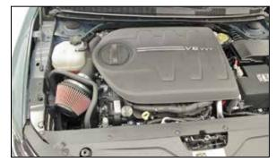
20. Reconnect the vehicle's negative battery cable. Double check to make sure everything is tight and properly positioned before starting the vehicle.
