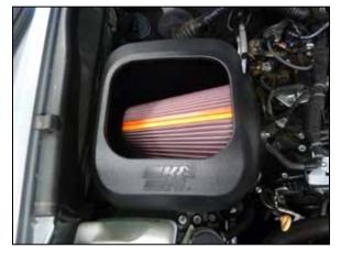
10. Install the air filter into the airbox.
