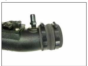
13. Slide hose with clamps on to the intake tube pass the bead like image shown. Tighten clamps using 5/16" socket or nut driver. **Note: Do not over tighten clamps.**
