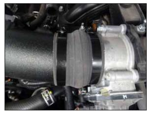
15. Now slide the hose onto the throttle body. adjust and rotate if necessary, and tighten all clamps. Tighten clamps using 5/16" socket or nut driver. **Note: Do not over tighten clamps.**
