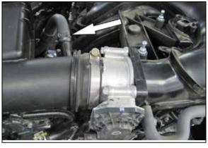
3. Release the spring clamp and disconnect the crank case vent hose from the factory intake tube.
