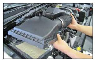
6. Release the two clips securing the upper air filter housing and then remove the intake tube and air filter hosing along with the factory air filter.
