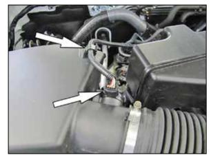
5. Disconnect the MAF sensor electrical connection and unhook the harness from the air filter housing.
