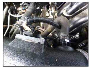
16. Connect the crank case vent hose to the barb fitting and secure using original spring clamp. Re-connect MAF sensor harness.
