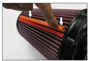
9. Attach the filter clips to the pleats on the air filter align and push down. Passenger side filters, place orange clip on top and red on bottom.
