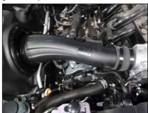
14. Install the intake tube assembly and position to air filter and throttle body.
