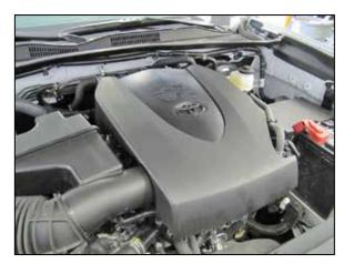
2. Lift up the engine cover to dislodge it from the mounting studs and then remove it from the vehicle.
