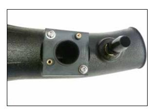
11. Install the provided 5/8" barb fitting into the K&N intake tube. Install the provided mass air sensor adapter onto the K&N intake tube using the provided hardware and gasket.
