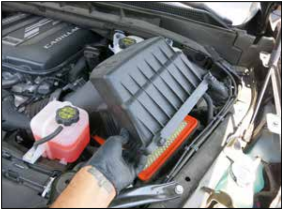
7. Loosen the bolts holding in the upper half of the air box and remove lid and air filter.
