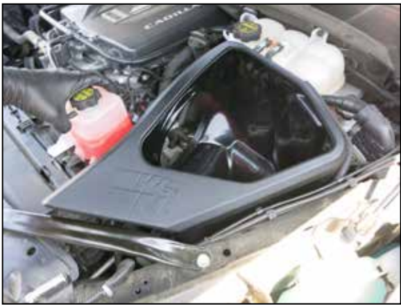
13. NOTE: Pre-assembled from the factory. Remove K&N Filter from airbox, Remove filter cap. Install the airbox into vehicle and position.
