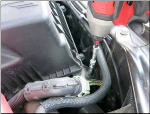
6. Remove the nut that secures the air filter housing. Save for later install. Unhook the wiring harness from the filter housing.
