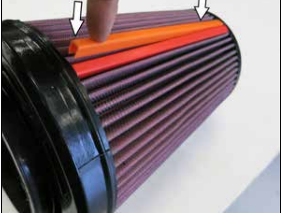
15. NOTE: Pre-assembled from the factory. Remove K&N Filter from airbox, Remove filter cap. Attach the filter clips to the pleats on the air filter align and push down. Driver side filter, place orange clip on top and red on bottom.
