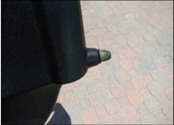
11. NOTE: Pre-assembled from the factory. Remove the OEM grommet from the air box and install to the K&N airbox mount.
