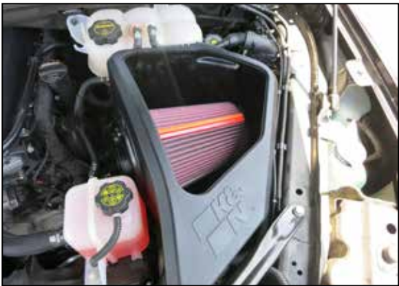
16. Install the air filter into the K&N airbox.
