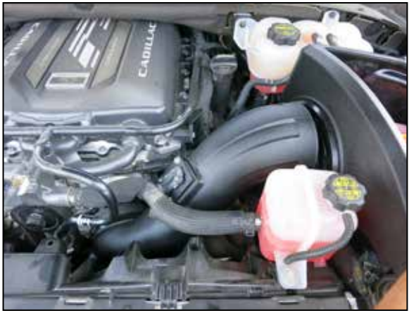
21. Install the intake tube to vehicle and position to air filter and hose on throttle body. Slide the straight hose onto the throttle body, Adjust for proper fit, and tighten all clamps.
