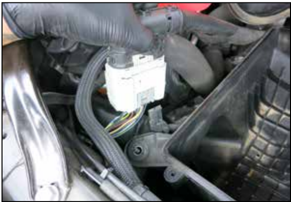
8. Using a small 90° pick or similar tool, release the locking tab that secures the wiring harness bulk connector to the air filter housing and then unhook the connector from the housing.
