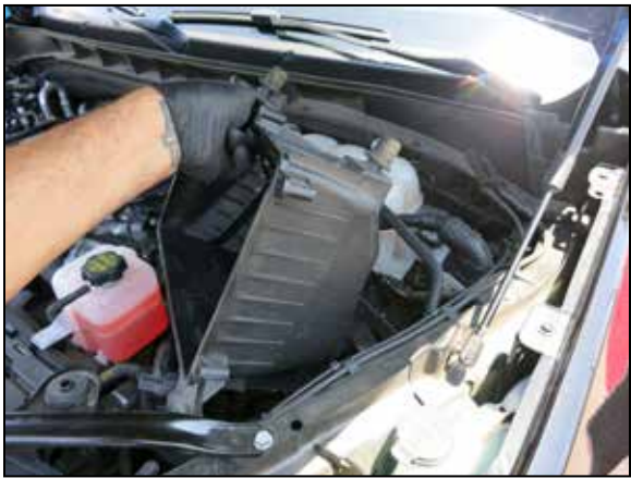
9. Now remove intake tube, and remove the lower part of the air box out of vehicle. Go slow and use caution to remove the housing. It is indexed into two holes in the rear with grommet. NOTE: Rubber grommets that can fall off easily and be lost. It is a tight fit but will come out without being forced. These grommets and nut will be reused in later steps. NOTE: K&N Engineering, Inc., recommends that customers do not discard factory air intake.
