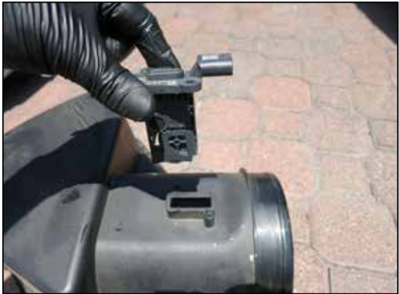
17. Carefully remove the MAF sensor from the OEM airbox.
