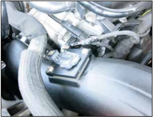
23. Connect the MAF sensor using provided harness extension.
