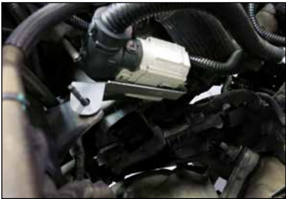
12. Install the provided bracket to the threaded stud air box mount. Slide the bulk connector to the bracket and secure. The K&N airbox will sit on top of this.
