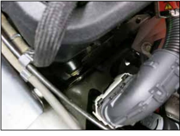
13. NOTE: Pre-assembled from the factory. Remove K&N Filter from airbox, Remove filter cap. Install the airbox into vehicle and position.
