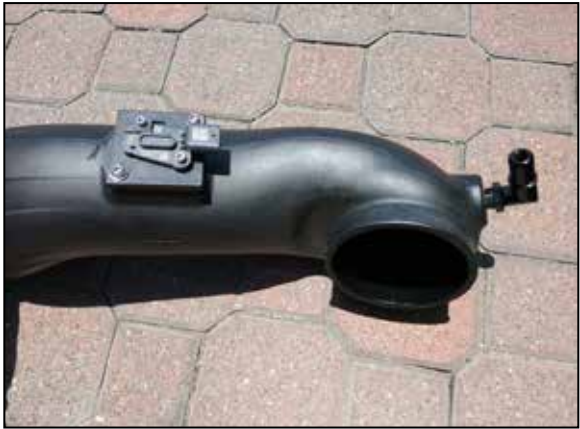
19. NOTE: Pre-assembled from the factory. Now install the MAF sensor into the intake tube and secure the sensor using provided hardware. NOTE: Make sure the sensor is going in the correct direction.
