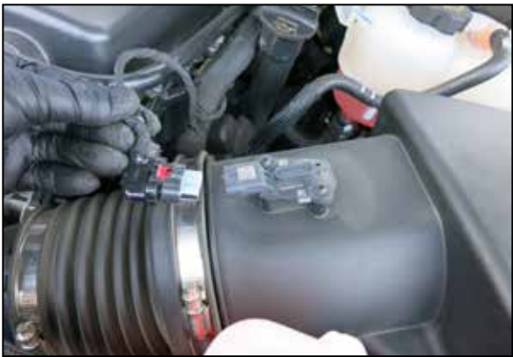
4. Disconnect the mass air sensor electrical connection.
