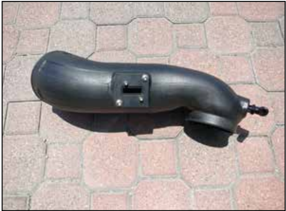
18. NOTE: Pre-assembled from the factory. Install the provided gasket onto the K&N® MAF sensor adapter and install to the intake tube like image shown. Secure and tighten using provided hardware. Install the provided 90 degree quick connect fitting into the K&N intake tube. NOTE: The quick connect fitting utilizes 3/8npt threads, thread the fitting in by hand and then tighten one revolution.
