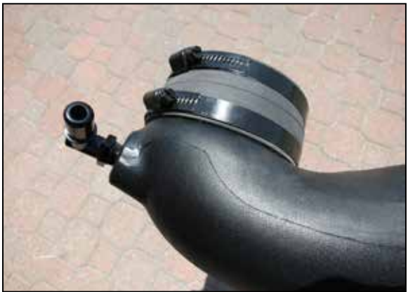
20. NOTE: Pre-assembled from the factory. Install the straight hose with clamps to the intake tube. Do not tighten clamps.
