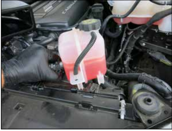
10. Loosen the bolt holding in the supercharger coolant tank and set to the side.
