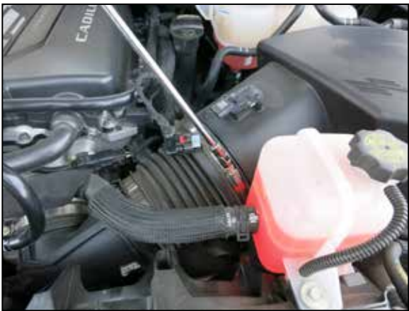
5. Loosen the hose clamps that secures the intake plenum to the air filter housing and to the throttle body. Disconnect the plenum connections at the air filter housing and then rotate the plenum counter clockwise to disengage the keyed mount and separate it from the throttle body.
