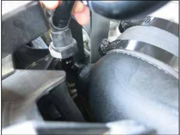
22. Re-connect the crankcase line. Make sure you hear a click to confirm it fits.
