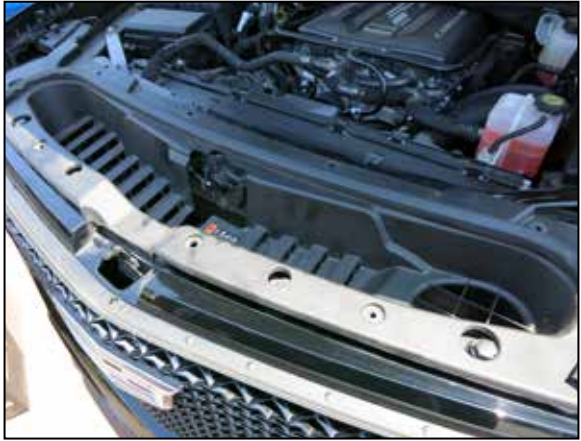
24. Reinstall the radiator valence and secure with the ten factory clips.
