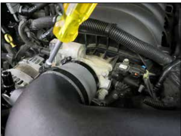
22. Adjust for proper fit, and tighten all clamps.
