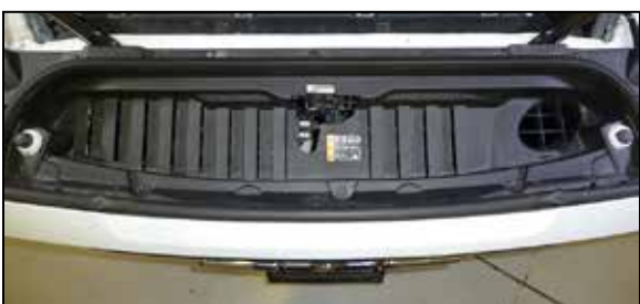
25. Reinstall the radiator valence and secure with the ten factory clips.
