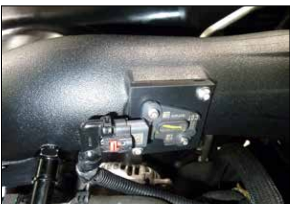
19. Reconnect the mass air sensor electrical connection.
