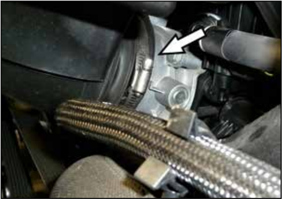
5. Loosen the hose clamp that secures the intake tube to the throttle body. Remove the intake plenum from the vehicle.
