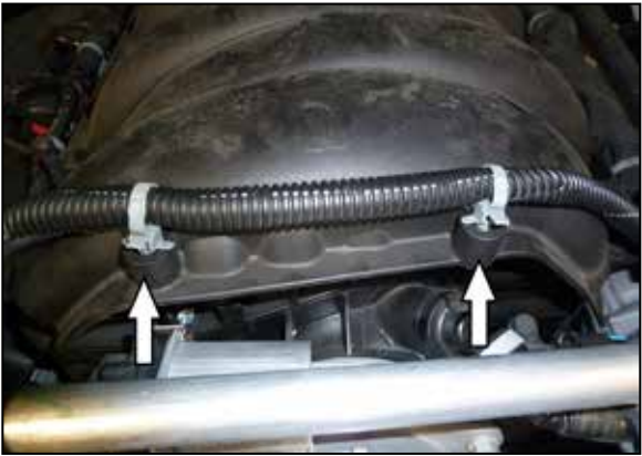
8. Disconnect the wiring harness from the intake manifold.
