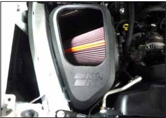
13. Install the K&N air filter into the K&N air filter housing.
