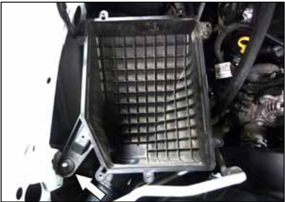
7. Remove the nut that secures the lower air filter housing and then lift the lower housing up to dislodge it from the mounting grommets and remove it from the vehicle. NOTE: The nut will be reused in the next step. NOTE: K&N Engineering, Inc., recommends that customers do not discard factory air intake.
