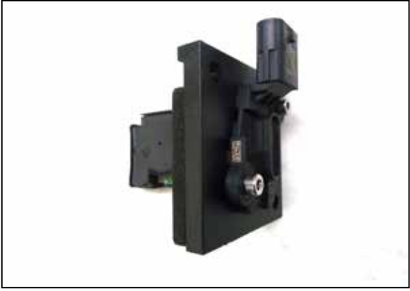
15. Remove the mass air sensor from the factory housing. Install the mass air sensor into the provided adapter and secure with the provided hardware. Install the adapter gasket onto the bottom of the adapter.
