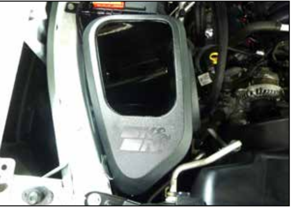
11. Install the K&N air filter housing into the vehicle so the mounting posts insert into the factory mounting grommets. Secure the air box with the factory nut from the previous step.
