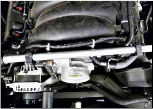
10. Secure the wiring harness and coolant pipe to the bracket as shown.
