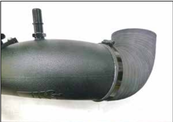
17. Install the elbow coupler onto the K&N intake tube as shown but do not fully tighten the hose clamp.
