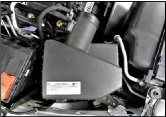
6. Remove the seven bolts that secure the upper air filter housing to the lower and then remove the upper housing and air filter from the vehicle.
