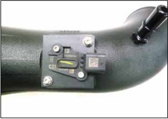
16. Install the mass air sensor assembly onto the intake tube using the provided hardware as shown. The sensor should be positioned as shown in the photo.
