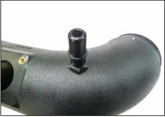
14. Install the provided 3/8npt quick connect fitting into the K&N intake tube as shown
