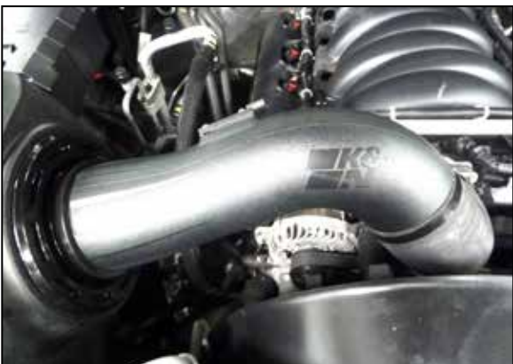
18. Install the K&N intake tube assembly into the K&N air filter and then connect the coupler to the throttle body, adjust the tube for best fit and then secure with the provided hose clamps.
