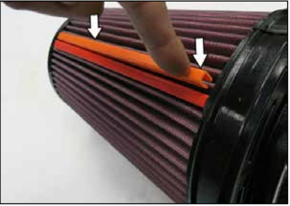
12. Attach the filter clips to the pleats on the air filter align and push down. Passenger side filters, place orange clip on top and red on bottom.
