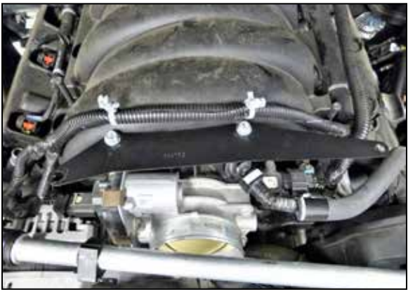
9. Install the provided mounting bracket onto the intake manifold using the provided hardware.
