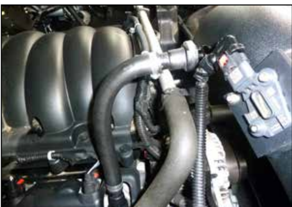
21. Install the CCV hose assembly onto the valve cover port and quick connect fitting installed into the K&N intake tube.
