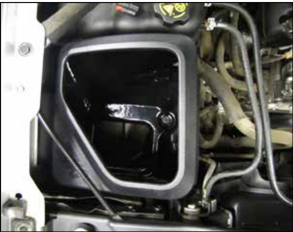
8. Install the K&N air filter housing so the fresh air intake passes through the opening in the inner fender and then secure the three factory bolts removed in step #7. NOTE: the wiring harness along the bottom the mounting plate may need to be adjusted for best fit.
