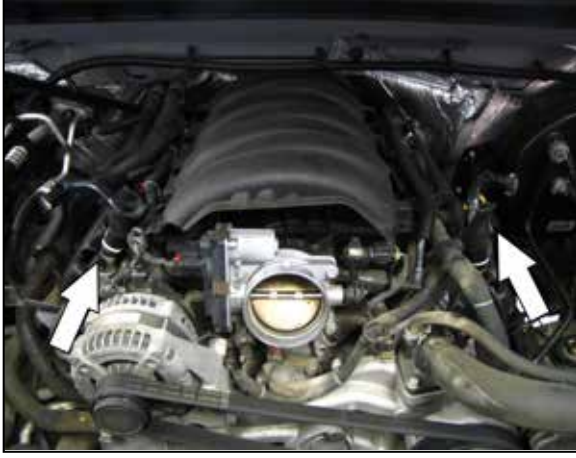
11. Depress the grey locking tabs and then remove the factory CCV hoses from the valve covers.
