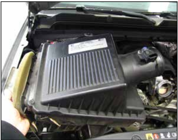
6. Lift the air filter housing up and then slide slightly to the right, then remove the housing from the vehicle.
