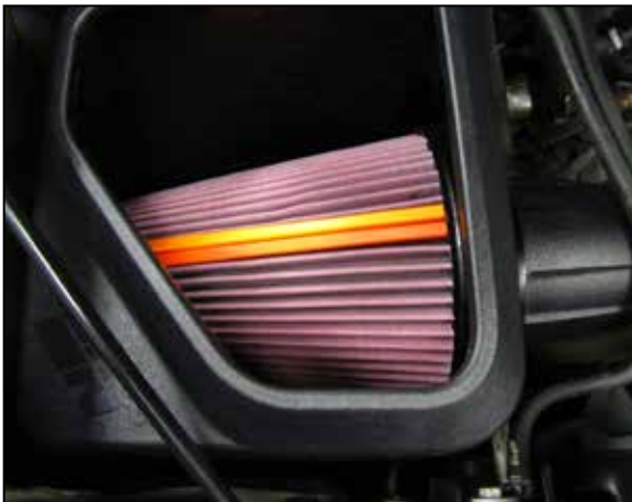
10. Install the K&N air filter into the K&N air filter housing.
