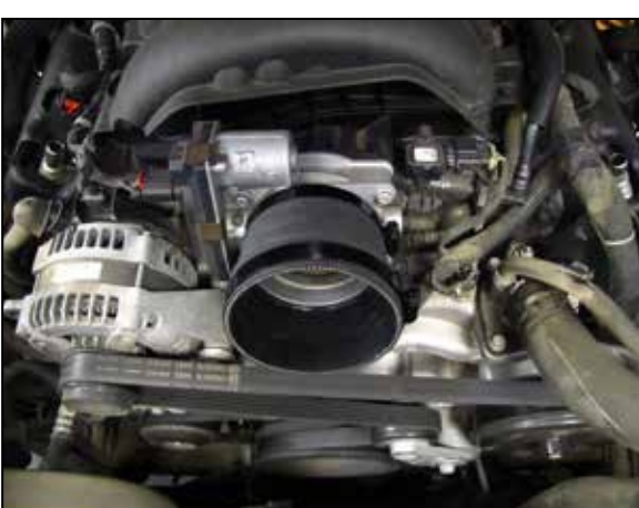
12. Install the step coupler (#08497) on 5.3L engines, hump coupler (#08418) on 6.2L engines and secure with the provided hose clamp. Tighten clamps using 5/16" socket or nut driver. Note: Do not over tighten clamps.
