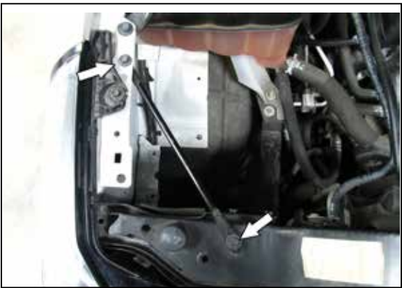
7B. Remove the two bolts that secure the fender to core support brace and remove the brace from the vehicle. NOTE: This brace will no longer be used on Cadillac Escalade & GMC Yukon vehicles only.
