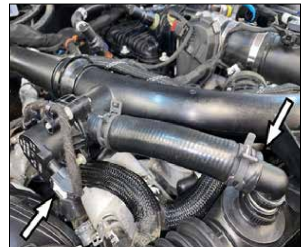
3. Release the BOV hose quick connect fitting and disconnect the BOV hose from the intake tube. Then disconnect BOV electrical connection and unhook the wiring harness from the mounting post.
