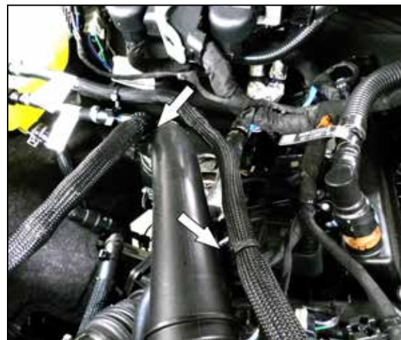
2. Disconnect the coolant hoses from the hot-side charge tube.
