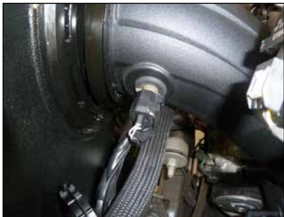
28. Reconnect the IAT sensor electrical connection.
