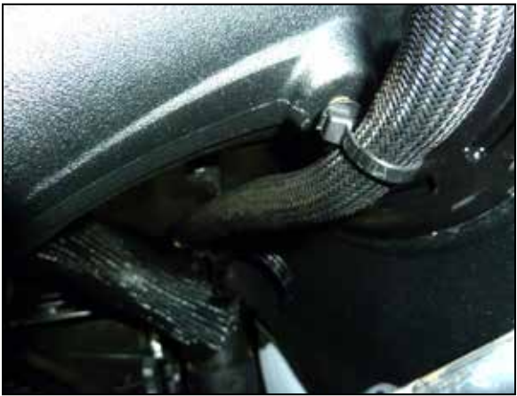
32. Secure the coolant hose to the intake tube on bottom with the provided mounting tie.
