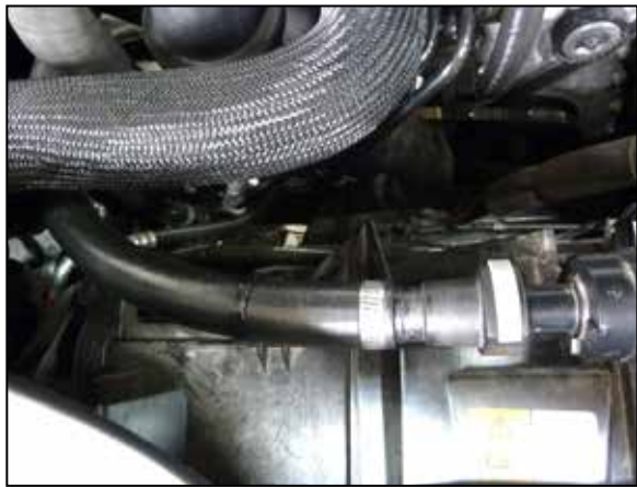
33. Install the provided BOV hose onto the intake tube and BOV valve and secure with the provided hose clamps.
