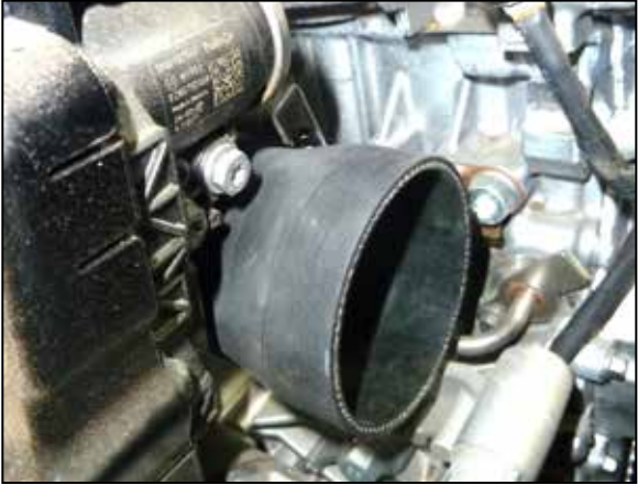
19. Install the provided step coupler onto the turbo inlet and secure with the provided hose clamp.
