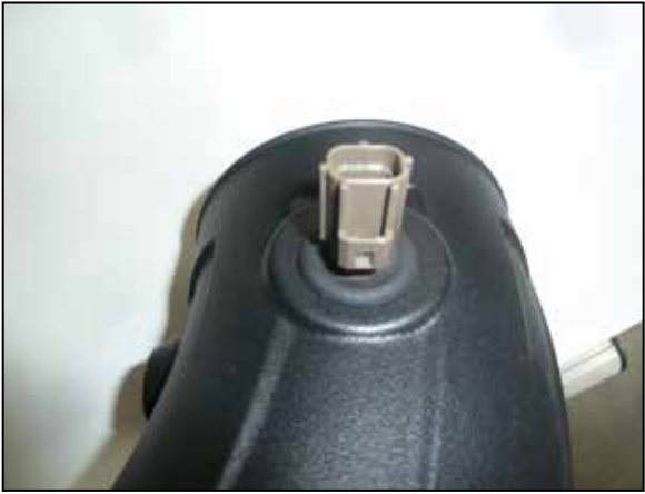
24. Remove the IAT sensor from the factory housing, remove the O-ring from the sensor and then install it into K&N intake tube using the provided grommet.
