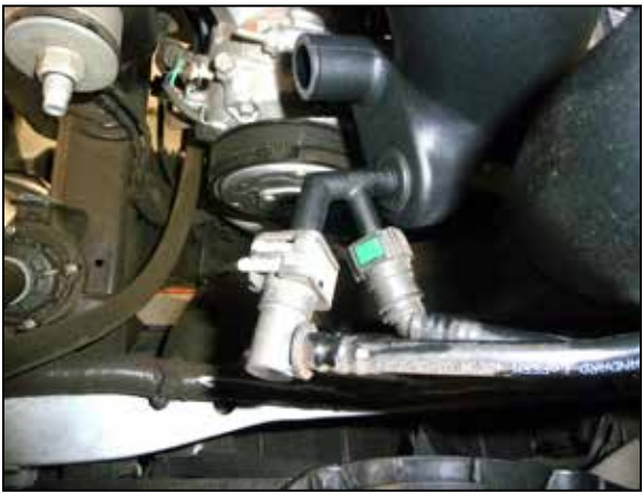
31. Connect the factory ejector lines to the ejector installed into the K&N intake tube.
