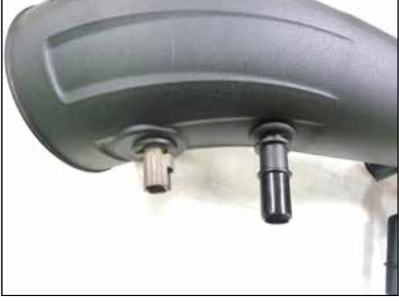
26. NOTE: Secondary vent line vehicles only, measure 3.0" from the center of the IAT sensor and drill a 7/8" id hole. Be sure to remove any debris or shavings after drilling. Install the vent fitting into the 7/8" id hole drilled into the K&N intake tube using the provided larger grommet.
