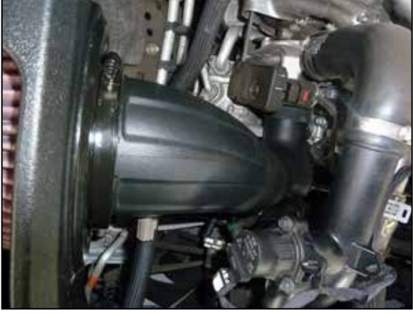
27. Install the K&N intake tube into the coupler at the turbo and then into the K&N air filter, align for best fit and then secure with the provided hose clamps.
