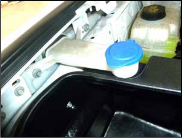
18. Reinstall the washer bottle filler neck using the factory hardware.
