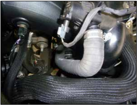
33. Install the provided BOV hose onto the intake tube and BOV valve and secure with the provided hose clamps.
