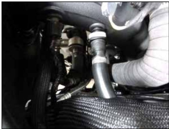
30. NOTE: Secondary vent line vehicles only, connect one end of the assembled hose to the factory quick connect fitting installed into the K&N intake tube. Then connect the other end to the quick connect hose above the radiator. If vehicle is only equipped with the CCV hose, this line will be extra, and not used.
