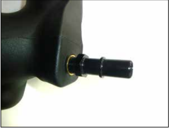
22. Install the provided quick connect fitting into the K&N intake tube as shown.
