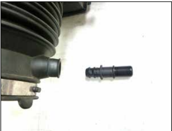
25. NOTE: Secondary vent line vehicles only, remove the vent fitting from the factory intake
