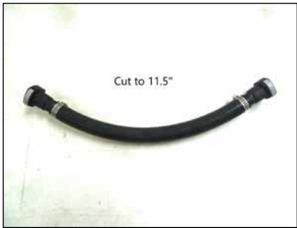
29. NOTE: Secondary vent line vehicles only, cut one of the provided vent hoses to 11.5" long, install the two provided straight quick connect couplers and secure with the provided hose clamps.
