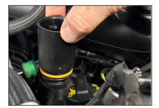
24. On some models, remove the oil filler neck extension and install the oil cap only.
