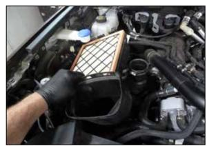
10. Remove the lower air filter housing and filter from the vehicle.
