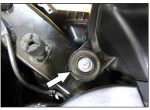
9. Remove the bolt that secures the fresh air duct to the core support and then remove the duct from the vehicle. **NOTE: This bolt will be reused.**
