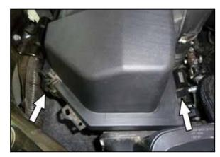
7. Release the two clips that secure the upper air filter housing and then remove the upper housing from the vehicle.
