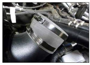
21.Install the provided coupler onto the open end of the passenger side intake tube, do not fully secure the hose clamp for the coupler currently. Tighten clamp using 5/16" socket or nut driver. **NOTE: Do not over tighten clamps.**
