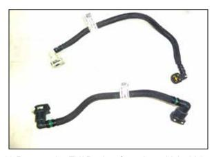
28 Remove the EVAP tubes from the vehicle. Using a hair dryer or similar heat source, warm the plastic EVAP tubes at the quick connect fittings to loosen the fitting enough that they will slip out from the tubes. NOTE: use caution to not melt the tubing or fittings.
