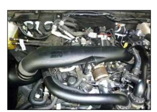
25. Install the K&N driver side intake tube into the factory turbo inlet fitting and then into the coupler at the passenger side intake tube, adjust the tube for best fit and then secure with the hose clamps. Tighten clamps using 5/16" socket or nut driver. **NOTE: Do not over tighten clamps.**
