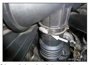
5. Loosen the hose clamp that secures the passenger side intake tube to the factory air filter housing.
