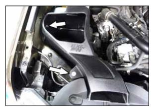
14. Install the K&N air filter housing into the vehicle so the mounting stud inserts into the factory mounting grommet and then secure it to the core support with the factory bolt removed during step #9. Secure the back of the K&N air filter housing with the factory bolt removed during step #11.
