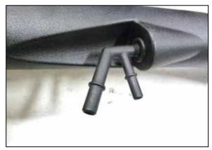
23. Install the K&N ejector fitting into the K&N driver side intake tube using the provided grommet. NOTE: Do not use excessive force with the ejector fitting as it is fragile.
