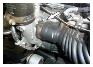
12.Loosen the hose clamp that secures the passenger side intake tube to the turbo and remove the tube from the vehicle.
