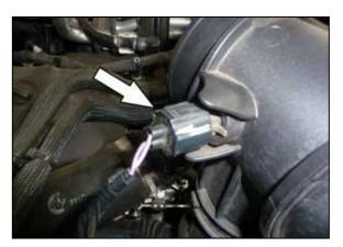
${\bf 6.\ Disconnect\ the\ IAT\ sensor\ electrical\ connection.}$
