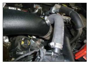
27. Install the provided BOV hose onto the valve and K&N intake tube and secure with the provided hose clamps. Tighten clamps using 5/16" socket or nut driver. **NOTE: Do not over tighten clamps.**
