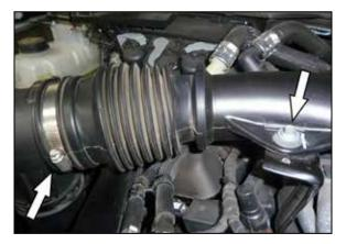
4. Loosen the hose clamp that secures the intake tube to the factory air filter housing. Remove the bolt that secures the intake tube to the mounting bracket on the engine and then remove the intake tube from the vehicle.
