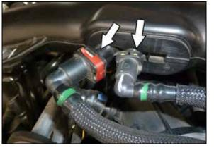
3. Remove the red locking clip, then disconnect the EVAP vent lines from the ejector fitting.
