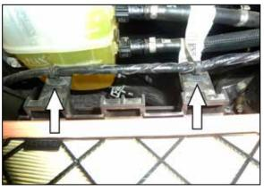
8. Disconnect the wiring harness from the lower air filter housing.
