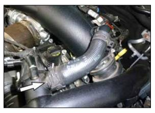
26. Release the spring clamp that secures BOV hose to the valve and then remove the hose from the vehicle.
