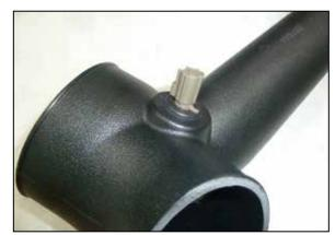
18. Remove the IAT sensor from the factory housing, remove the O-ring from the sensor and then install the sensor into the K&N passenger side intake tube using the provided grommet.
