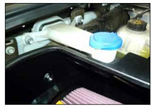
17. Reinstall the washer bottle filler neck and secure with the factory mounting bolts removed during step #11.
