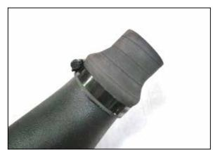
19. Install the reducer coupler onto the K&N passenger side intake tube and secure with the provided hose clamp. Tighten clamp using 5/16" socket or nut driver. **NOTE: Do not over tighten clamps.**
