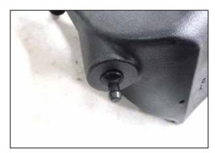
13. Install the provided mounting stud onto the K&N air filter housing using the provided hardware.
