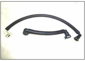
29. Install the EVAP quick connect fittings from the previous steps into the provided EVAP hoses.
