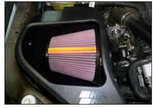
16. Install the K&N air filter into the K&N air filter housing.
