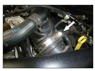
2. Loosen the hose clamp that secures the intake tube to the turbo inlet, then release the BOV fitting from the intake tube.
