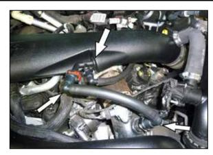
30. Install the EVAP lines onto the ejector fitting in the K&N intake tube and then connect the open ends to the factory ports.
