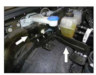
11. Remove the two bolts that secure the washer bottle filler neck to the bottle and remove the filler neck. NOTE: The filler neck will be reinstalled and secured with the factory bolts in a later step. Remove the lower airbox bracket and save bolt. NOTE: This bolt will be reused.
