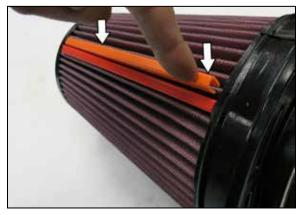
15. Attach the filter clips to the pleats on the air filter align and push down. Passenger side filters, place orange clip on top and red on bottom.
