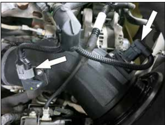
20. Reconnect the mass air sensor and IAT sensor electrical connections. Cable-ties provided to secure harness if necessary.
