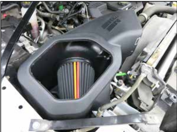
18. Now install the K&N air filter housing into the vehicle so the mounting studs insert into the mounting grommets, at the same time aligning the intake tube into filter.
