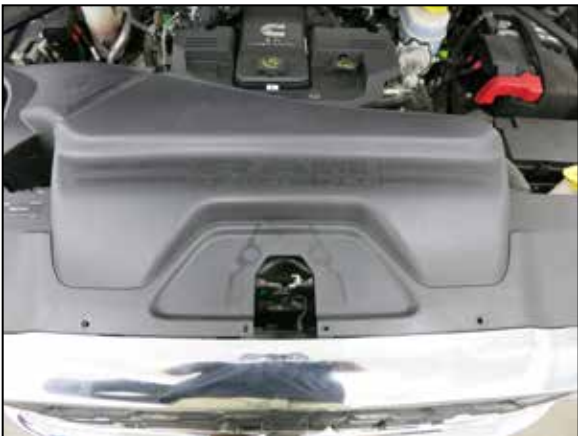
22. Re-install the upper core support plastic cover.
