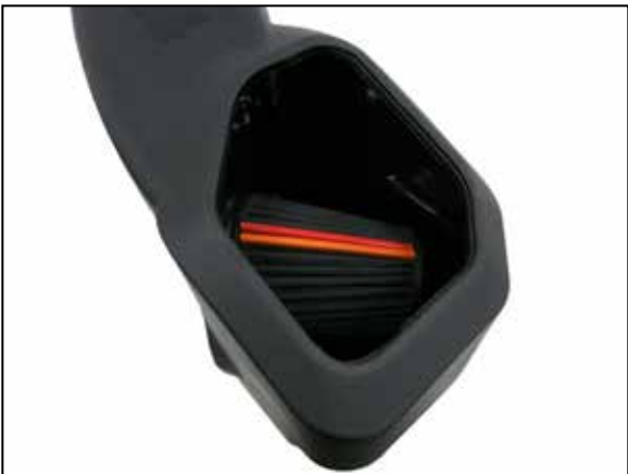
17. Install the K&N air filter into the K&N air filter housing.
