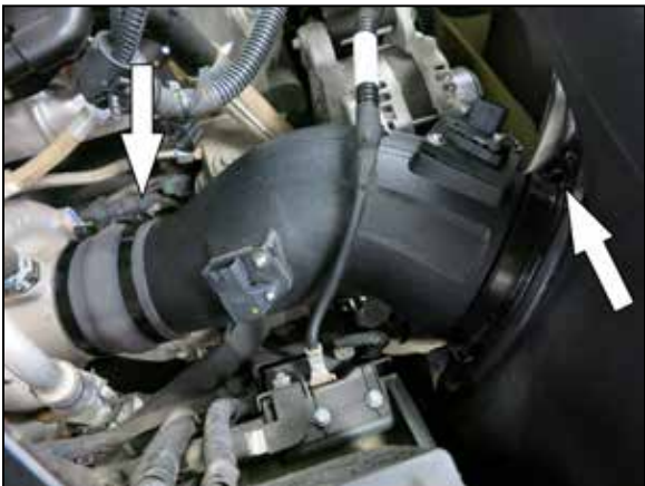
19. Once intake tube is positioned, tighten remaining 2 clamps.
