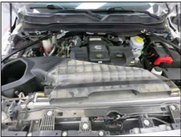
21. Re-install the fresh air duct and secure.
