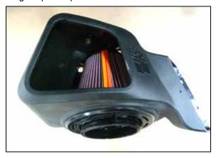
11. Install the K&N air filter into the K&N air filter housing as shown.
