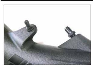
16. Install the provided mounting stud onto the K&N intake tube using the provided hardware. Install the CCV vent fitting provided into the K&N intake tube.
