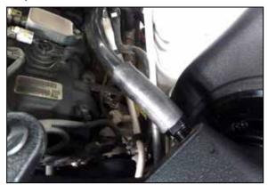
18. Install the provided CCV hose onto the factory CCV pipe and then connect it to the CCV fitting installed into the K&N intake tube.
