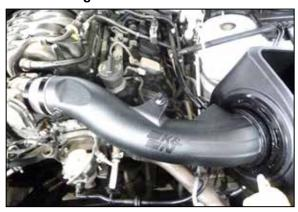
17. Install the K&N intake tube into the air filter and then into the coupler at the throttle body, adjust for best fit and then secure with the provided hose clamps.
