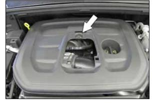
2. Lift the inspection cover and remove the bolt that secures the decorative engine cover. Then remove the decorative engine cover from the vehicle. NOTE: The cover is also secured by four mounting studs and grommets
