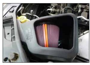
12. Install the K&N air filter housing assembly into the vehicle so the mounting studs insert into the grommets.
