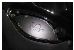
19. During inclement weather, install the provided heat extractor vent block-off if the vehicle is equipped with heat extractor vents. On Dodge vehicles, remove the two bolts that secure the driver side vent. Install and secure the provided block-off and securewith the factory hardware.
