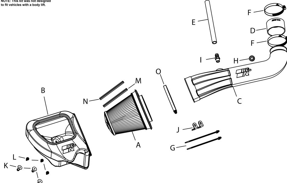
Α AIR FILTER RU-5303 HOSE CLAMP; #52 BLK 08610KA MOUNT; PLASTIC AIRBOX 3 8-186-1 **AIRBOX** ZIP TIE; 8" TREE PUSH-MNT BOLT; M6-1 X 12, HEX В 087635 G 1-127 1-2110 С TUBE 087636 GROMMET; 9/16"ID KITGRMT02 CLIP; SNAP-ON, RED 088222 HOSE; 3.25"ID X 2"L 08690 FITTING; 5/8" BARB TO 3/8"NPT 82635 CLIP; SNAP-ON, ORANGE 088223 HOSE; 5/8"ID X 10"L BRACKET; "L" HOSE CLAMP; #88 BLK 5-7010 070066A 0 KITHS88K
