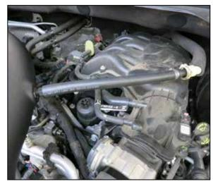
15. Connect the CCV hose quick connect fitting into the factory CCV fitting.
