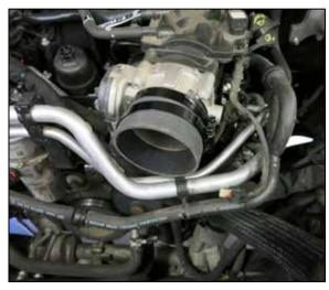
8. Install the provided coupler onto the throttle body with the hose clamps. Tighten clamps using 5/16" socket or nut driver.
