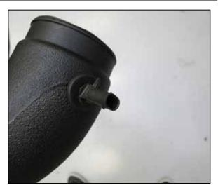
13. Remove the IAT sensor from the factory intake plenum, remove the O-ring from the sensor and then install it into the K&N intake tube with the provided grommet.
