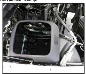
7. Install the K&N air filter housing into the vehicle so the mounting posts protrude through the mounting grommets.
