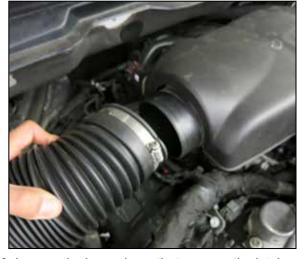
3. Loosen the hose clamp that secures the intake hose to the intake plenum and then disconnect the hose.
