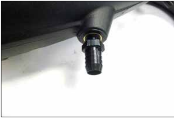
19. Install the provided barb fitting into the K&N intake tube. NOTE: The quick connect fitting utilizes 3/8npt threads, thread the fitting in by hand and then tighten one revolution.
