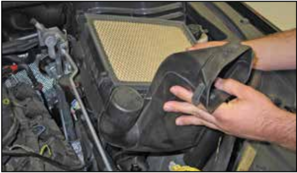
9. Lift up the lower airbox to dislodge it from the mounting grommets and then remove the lower airbox from the vehicle. Some vehicles may have a power steering line attached to the air box than will need to be unhooked.
