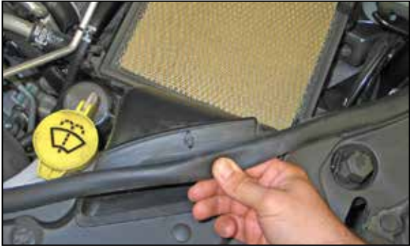
8. Unhook the sealing trim from the fresh air intake scoop and keep clip.
