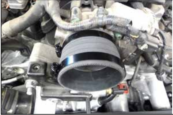
17. Install the hose with clamps to the throttle body and tighten clamp on throttle body only. Tighten clamps using 5/16" socket or nut driver. Note: Do not over tighten clamps.
