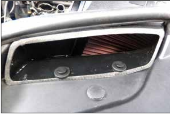
16. Secure the front of the airbox using provided push clips.
