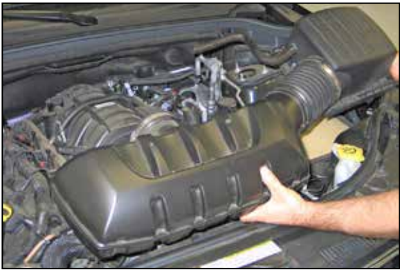
7. Remove the upper airbox and intake tube assembly.
