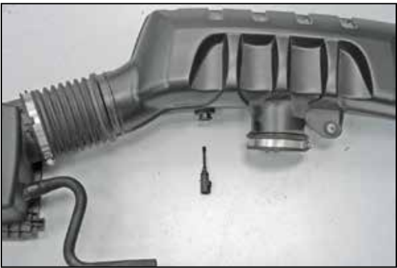
11. Release the locking tab and then remove the inlet air temperature sensor from the factory intake tube by twisting counter clockwise. NOTE: The inlet air temperature sensor is very fragile; take care to avoid damage while handling the sensor.
