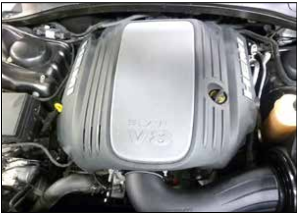
19. Reinstall the factory engine cover.
