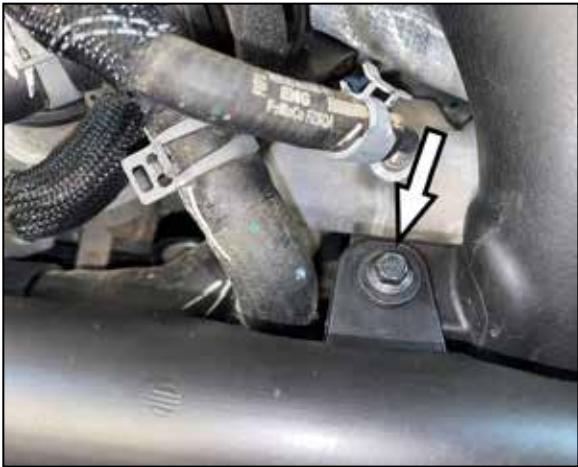
6. Remove the bolt shown that secures the drivers side intake tube to the cold-side charge tube and then remove the drivers side intake tube from the vehicle.
