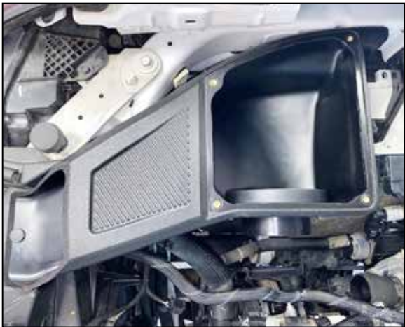
14. Set the K&N air filter housing into position and secure with the factory push-pin and the provided bolt.
