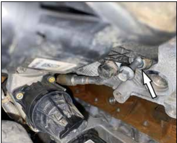
11. Reinstall the intake tube mounting bolt into the original location and tighten.
