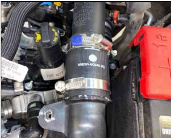
5. Loosen the hose clamps the secure the driver's side intake tube.
