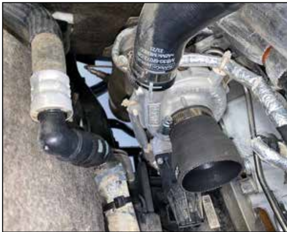
12. Install the provided step coupler onto the passenger side turbo inlet and secure with the provided hose clamp.
