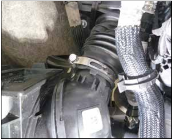
9. Loosen the hose clamp that secures the passenger side intake hose to the air filter housing and then remove the factory air filter housing from the vehicle.
