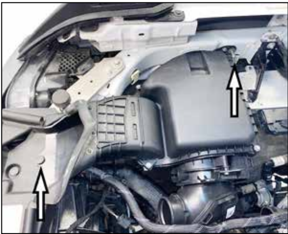
7. Remove the push-pin that secures the fresh air inlet. Remove the air filter housing mounting bolt.
