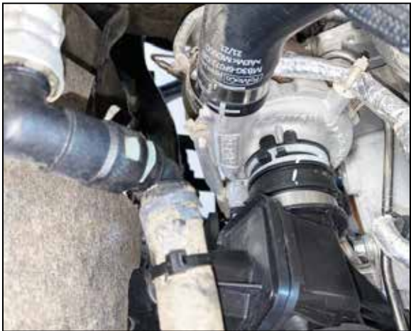
10. Remove the bolt on the bottom side of the passenger side intake tube that secures the tube to the engine. Then Release the spring clamp that secures the intake tube to the turbo and remove the passenger side intake tube. NOTE: The spring clamp is difficult to release with the tabs positioned towards the bottom of the turbo inlet.
