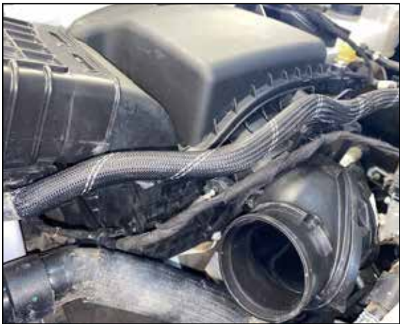
8. Unhook the wiring harness and coolant hoses from the air filter housing.
