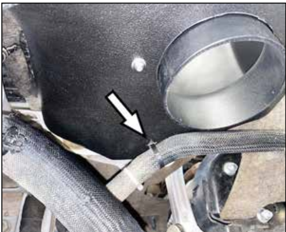
15. Secure the lower coolant hose to the air filter housing.
