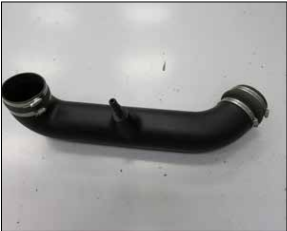
20. Install the couplers onto the K&N intake tube and secure with the provided hose clamps.
