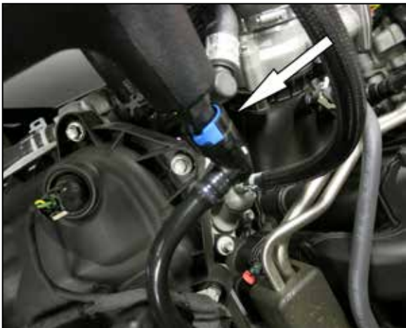
22. Connect the factory CCV hose to the quick connect fitting installed into the K&N intake tube.
