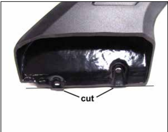
12B. In these cases, it will be necessary to trim the mounting tabs as shown using a hack saw or similar tool.
