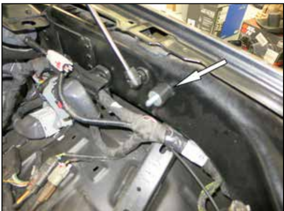
11. Install the provided rubber mounted stud into the inner fender at the air filter housing mounting location.
