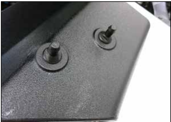
9. Install the provided mounting studs onto the K&N lower air filter housing using the provided hardware.
