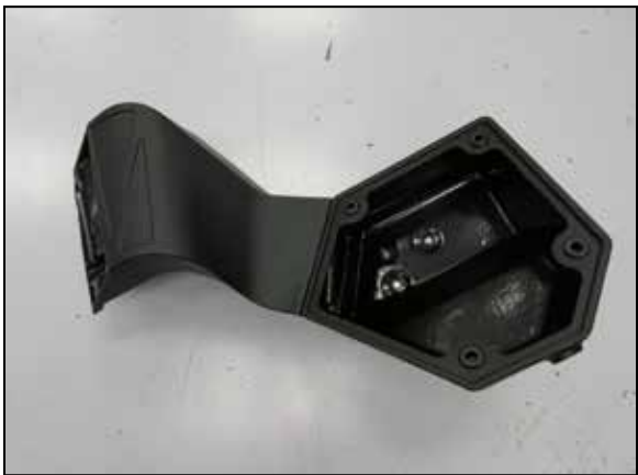
10. Install the K&N fresh air duct onto the K&N lower air filter housing using the provided hardware.
