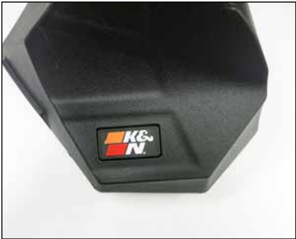
15. Snap the K&N badge into the upper air filter housing.
