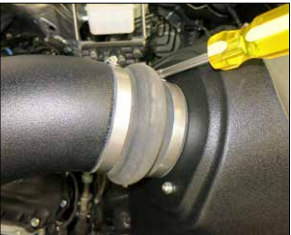
21. Install the K&N intake tube into the onto the throttle body and filter adapter, adjust for best fit and then secure with the provided hose clamps.
