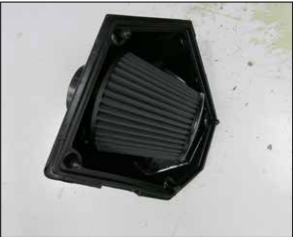
17. Install the K&N air filter onto the adapter and secure with the provided hose clamp.
