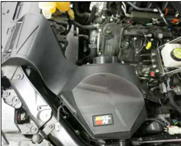
18. Install the upper housing assembly onto the lower housing so the mounting posts insert into the grommets.
