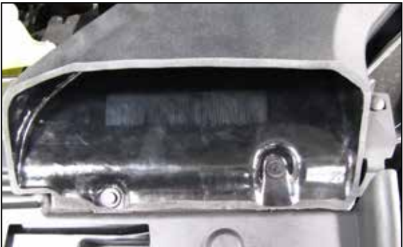
12C. Once the tabs are trimmed flush with the fresh air duct the air filter housing can be installed back into position, pushed down and the locking pins installed as intended.
