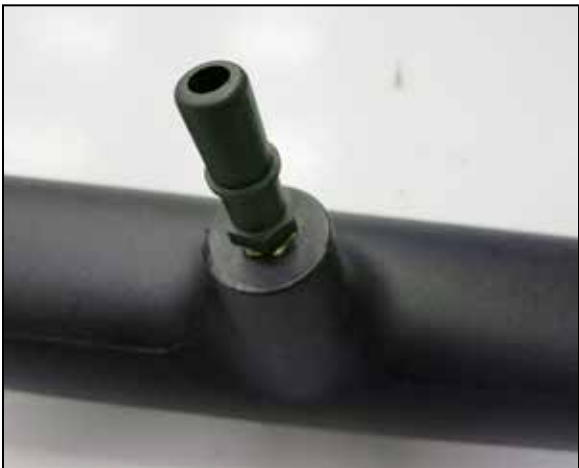
19. Install the provided CCV quick connect fitting into the K&N intake tube.
