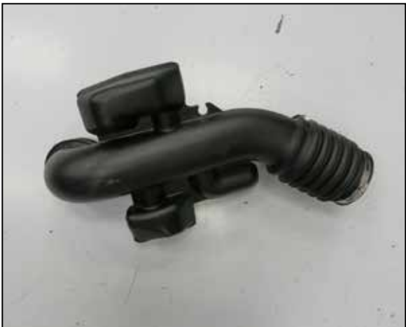
4. Remove the intake tube from the vehicle.
