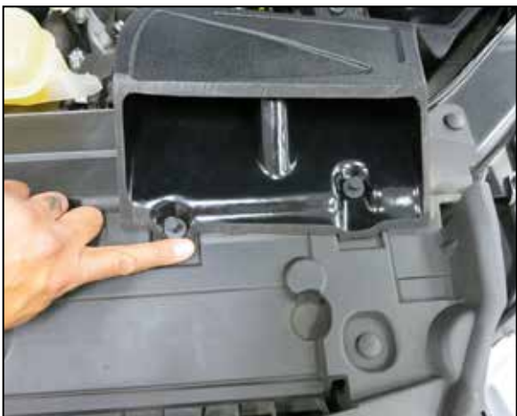
14. Secure the fresh air intake duct with the provided push pins.
