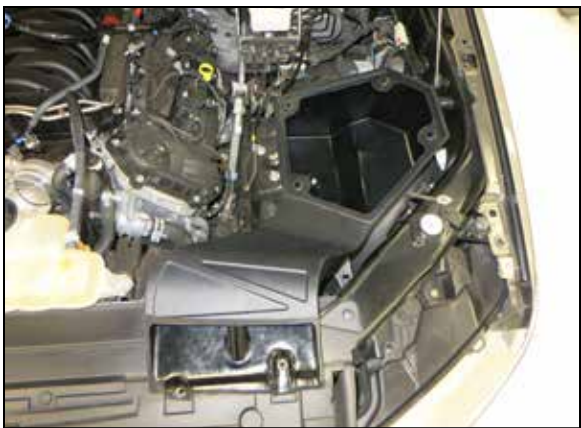
12. Install the K&N lower air filter housing assembly into the vehicle.
