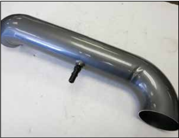
16. Install the provided quick connect fitting into the intake tube as shown.
