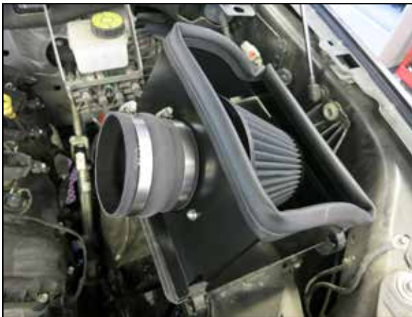
15. Install the provided hump hose onto the filter adapter and secure with the provided hose clamp.
