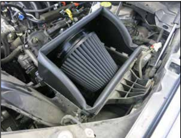
14. Install the Heat shield/Filter assembly onto the lower air filter housing and secure with the factory retaining clips.
