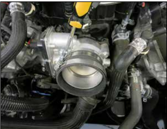
13. Install the provided straight coupler onto the throttle body and secure with the provided hose clamp.
