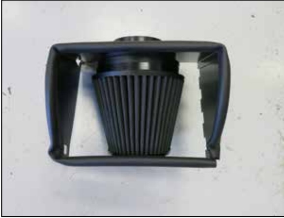
11. Install the air filter onto the filter adapter and secure with the provided hose clamp.
