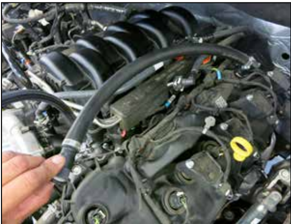
12. Install the CCV assembly onto the engine. NOTE: the 90deg fitting will be attached to the engine.
