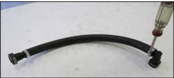
7. Assemble the provided CCV hose assembly using the hose, fittings, and clamps.
