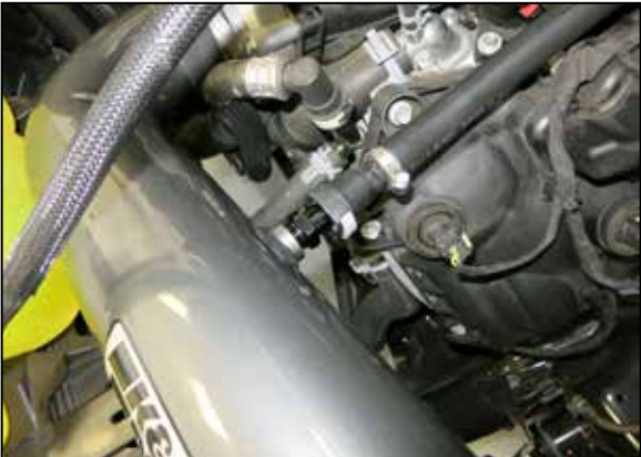
18. Connect the CCV hose to the quick connect fitting installed onto the intake tube.
