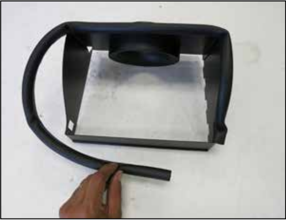
10. Install the bulb edge trim to the top of the heat shield as shown. Some trimming of the edge trim will be necessary.
