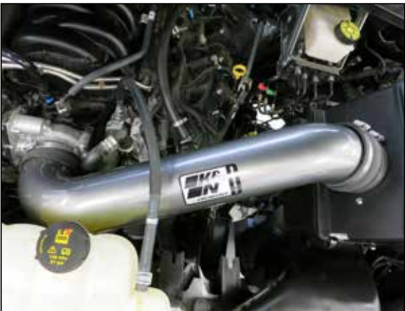
17. Install the Intake tube into the coupler at the throttle body and then into the coupler at the filter adapter, adjust the tube for best fit and secure with the provided hose clamps.
