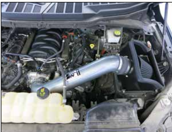
19. Reconnect the vehicle's negative battery cable. Double check to make sure everything is tight and properly positioned before starting the vehicle.
