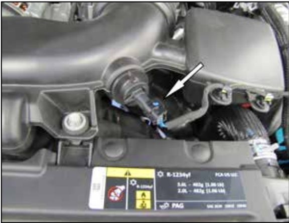
2. Disconnect the inlet air temp electrical connector.
