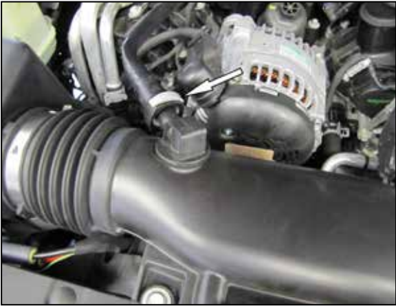
3. Disconnect the crank case vent line.
