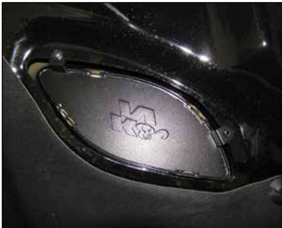
26. Install the block off and secure with the factory hardware. Jeep models will use the EPDM block off.
