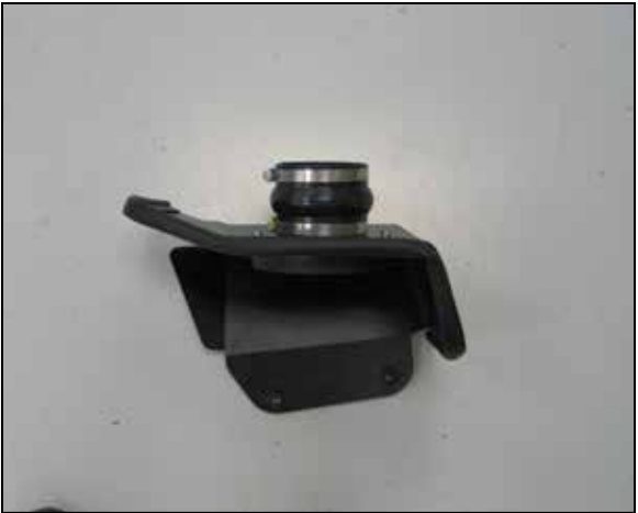
14. Install the provided silicone hump hose (084057) onto the filter adapter and secure with the provided hose clamp.
