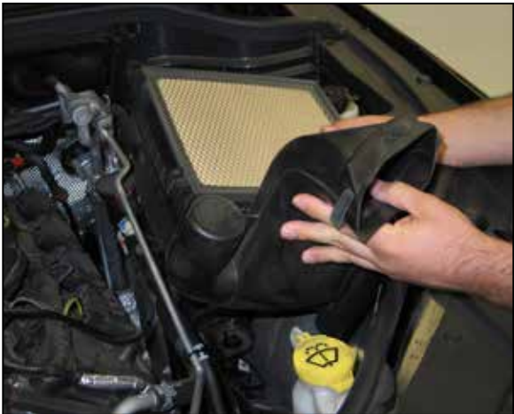
9. Lift up the lower airbox to dislodge it from the mounting grommets and then remove the lower airbox from the vehicle. NOTE: K&N Engineering, Inc., recommends that customers do not discard factory air intake.
