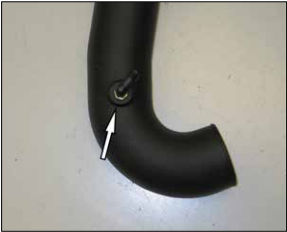
21. Install the 90° npt fitting into the K&N intake tube as shown.
