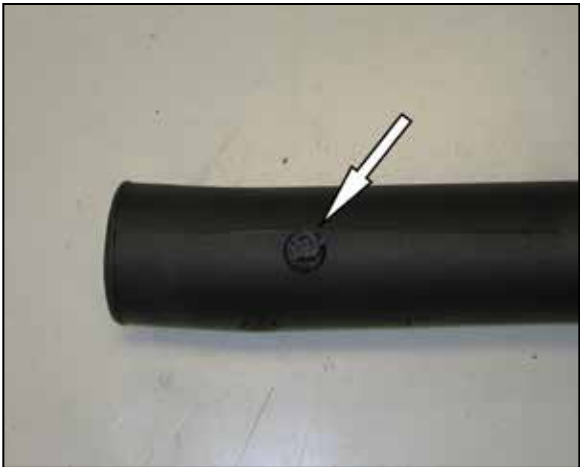
20. Install the inlet air temperature sensor into the K&N intake tube. NOTE: Be sure to remove the O-ring from the inlet air temperature sensor before installing.
