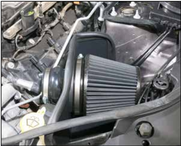
16. Install the K&N filter onto the adapter and secure with the provided hose clamp.
