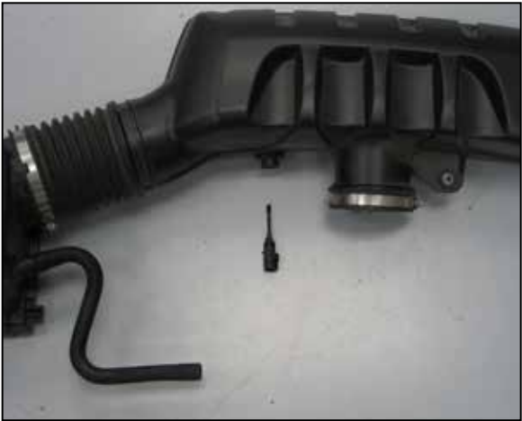
18. Release the locking tab and then remove the inlet air temperature sensor from the factory intake tube by twisting counter clockwise. NOTE: The inlet air temperature sensor is very fragile; take care to avoid damage while handling the sensor.
