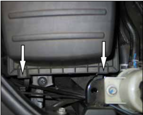
6. Release the two upper airbox retaining clips.
