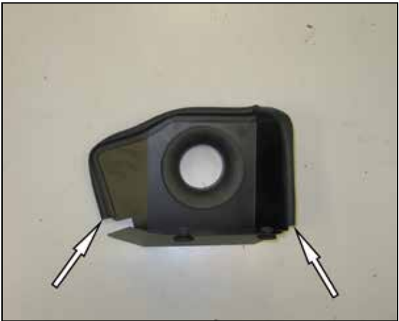
13. Install the provided edge trim onto the heat shield as shown. NOTE: Some trimming of the edge trim will be necessary.
