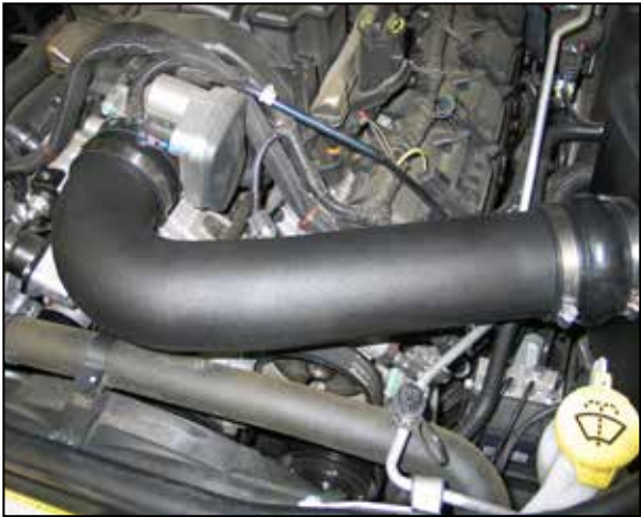
22. Install the K&N intake tube into the silicone hump hose and then into the silicone hose at the throttle body, secure the intake tube with the provided hose clamp.
