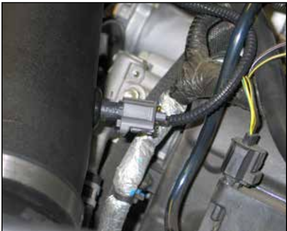
23. Install the crankcase vent hose onto the 90° vent fitting and then attach the open end to the valve cover port. Connect the inlet air temperature sensor extension harness into the factory electrical connection and then connect the other end into the inlet air temperature sensor as shown.
