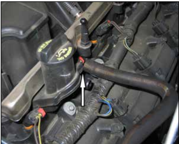
5. Disconnect the crankcase vent hose from the port on the valve cover.
