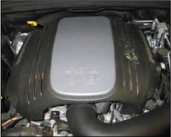
24. Reinstall the engine cover.
