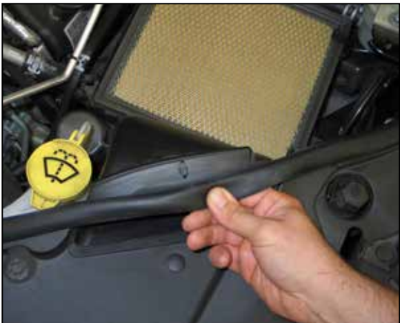
8. Unhook the sealing trim from the fresh air intake scoop.
