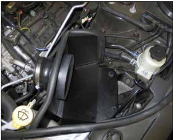
15. Set the heat shield into the vehicle so that the mounting grommets slide over the factory airbox mounting studs.
