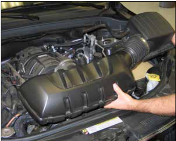
7. Remove the upper airbox and intake tube assembly.
