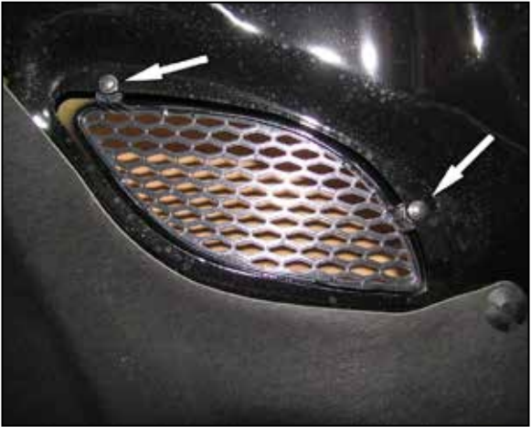
25. On models with heat extractor vents installed in the hood it is recommended to install the provided extractor block off plate. On Dodge vehicles, remove the two bolts holding in the grill.
