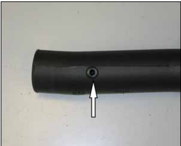
19. Install the provided grommet into the K&N intake tube as shown.
