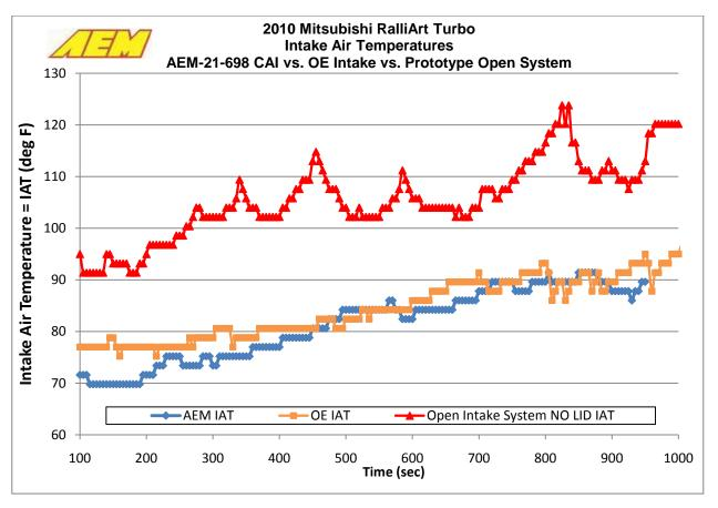
In developing this intake system, we also tested several combinations of tube diameters, DRYFLOW air filter sizes, and sealed or unsealed airboxes to determine the best solution for the RalliArt. Our goal was to maximize the amount air flow to the turbo and minimize intake air temperatures, all while maintaining the proper fuel trims to stay within the stock MAF calibration. The final design yielded a substantial increase in flow over the stock intake system as seen in Figure 2:
